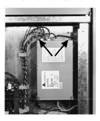
Figure 5-4 Mounting Screws (24/42 V power supply shown)
