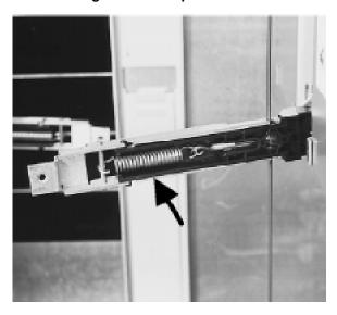
Figure 5-31 Two Ends of the Slave Rope in the Tensioner
