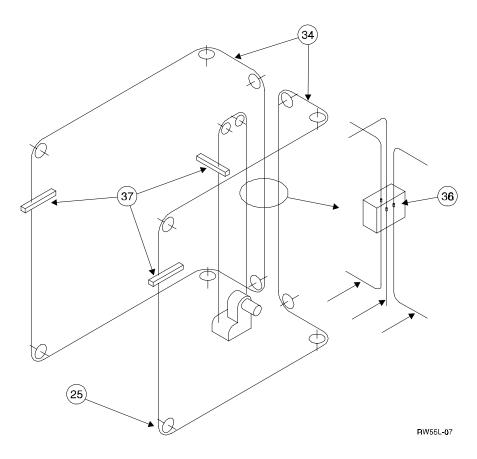
Figure 5-44 Jukebox Pulley and Rope Diagram
