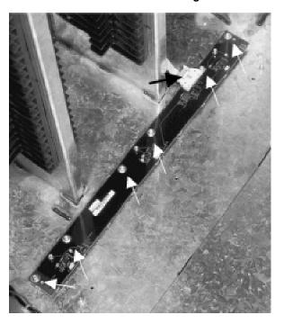
Figure 5-42 Vertical Path Clear PCA Mounting Screws
