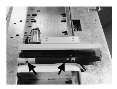
Figure 5-6 Mailslot Assembly Mounting Screws
