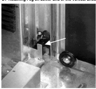
Figure 5–24 Retaining Peg on Lower End of the Vertical Encoder Strip
