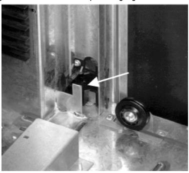
Figure 5-19 Vertical Encoder Strip Mounting Peg
