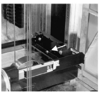
Figure 5–20 Removing the Visual Locator Bracket
