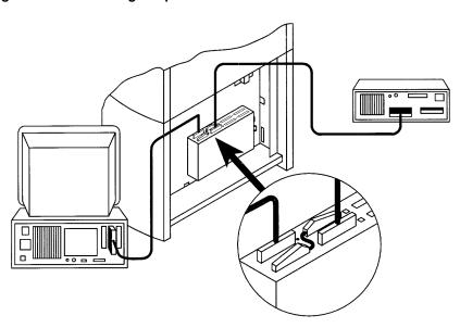
Figure 3-4 Connecting Peripheral Devices with Bus 1
