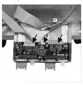
Figure 5-39 SCSI Repeater / LUN Converter PCA
