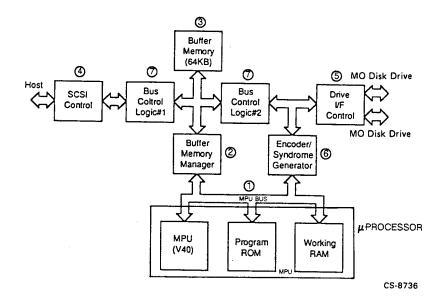
1. Microprocessor Module - This module (MPU) includes a V40 MPU, a 64K byte programmable ROM (PROM), and a 32K byte working RAM on the MPU bus. This module controls and manages the other modules in the SCSI controller and in the disk drive section. Another major function is to correct errors in the data that was read.
