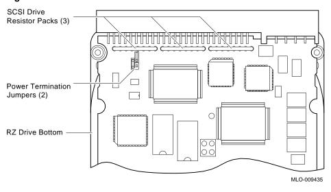
When adding a SCSI 3 1/2-inch disk drive to the DEC 4000 AXP system, remove the three resistor packs and two power termination jumpers shown in Figure 1 to avoid bus problems.
