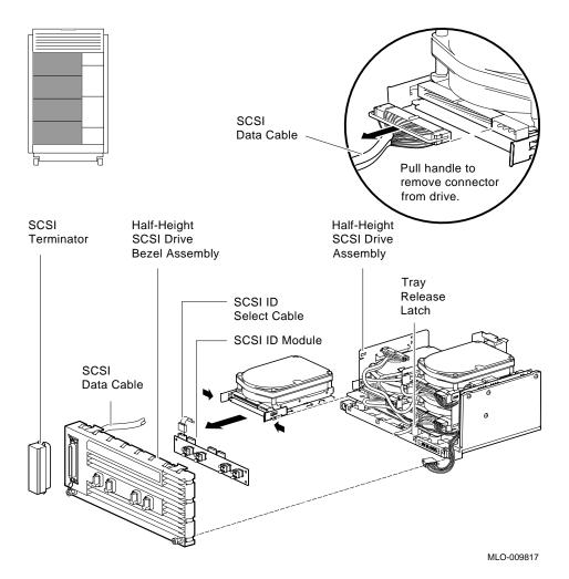
Figure 3 RZ-Series 3 1/2-Inch Fast SCSI Storage Assembly
