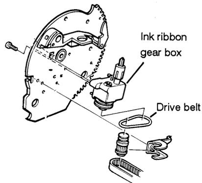
Figure 36 Removing the ink ribbon gear box. This figure is intended for parts identification only. No other parts need to be removed or loosened
