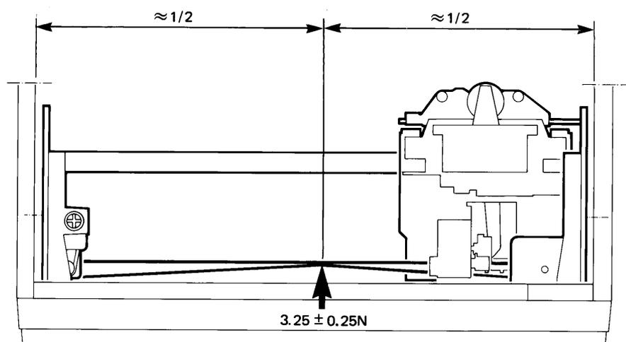
Figure 3-8a Checking the carriage drive belt tension
