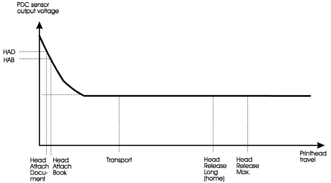
Figure 2-21 PDC sensor output voltage
