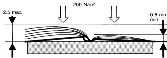
Figure 1-8 Measuring passbook thickness
