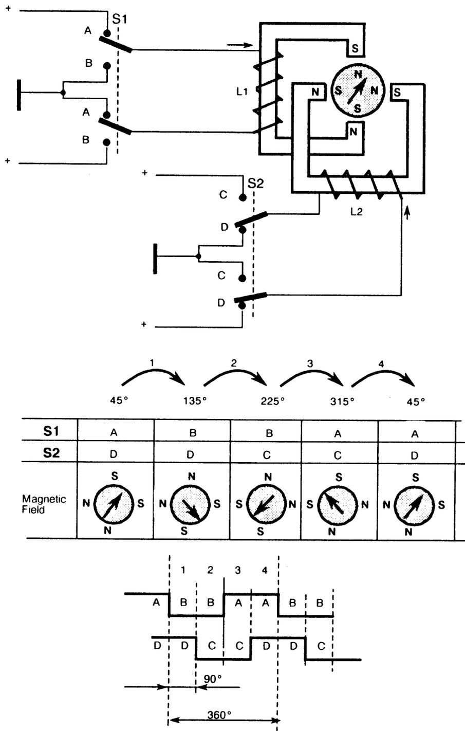
Figure 2-35 Simplified description of the stepper motor function
