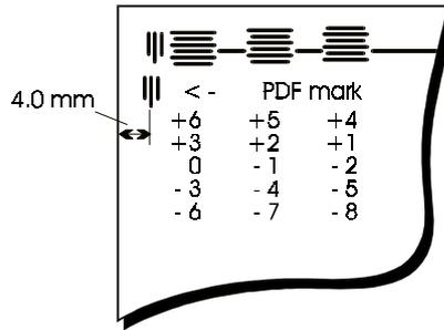
Figure 3-21 Measuring the PDF offset correction
