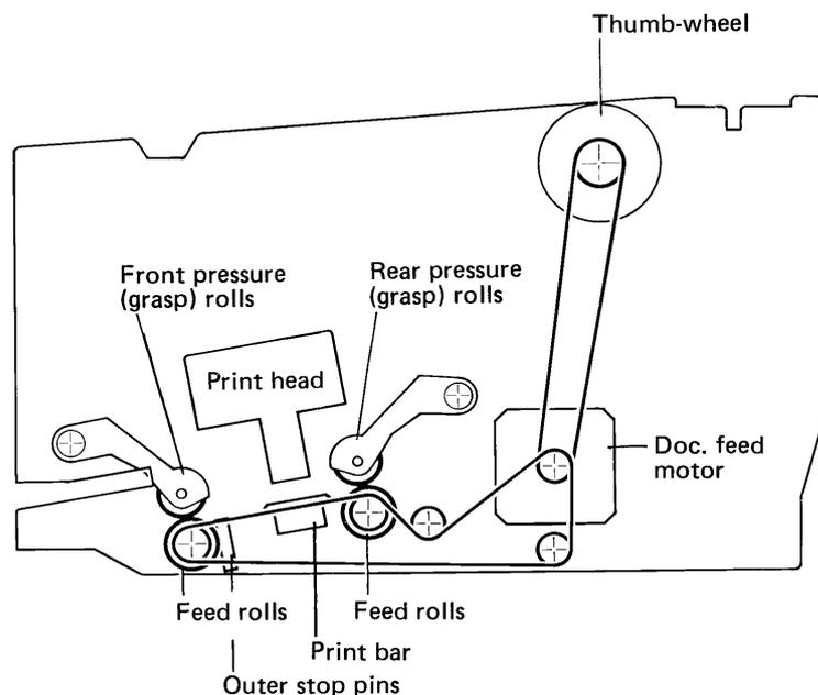
Figure 2-1 Document feed mechanism
