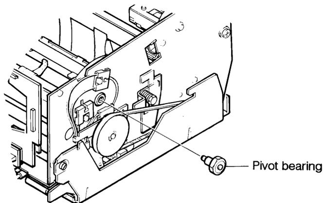
Figure 3-32 Removing the right side pivot bearing
