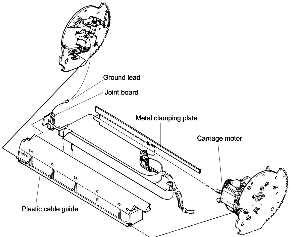
Figure 3-35 Removing the carriage motor (this figure is intended for parts identification only)
