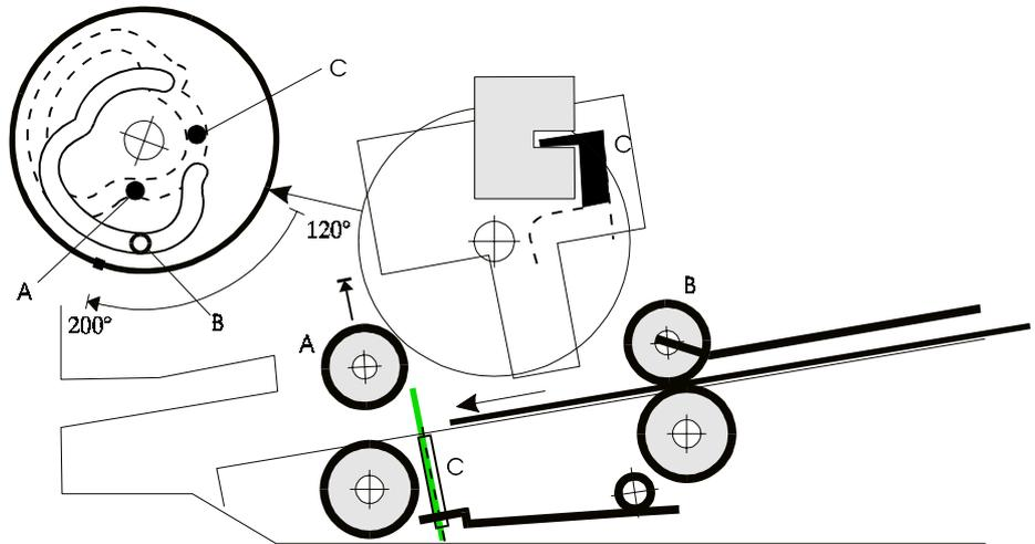
Figure 2-8 The front pressure rolls raised to let the document pass on its way out
