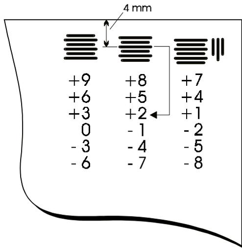
Figure 3-18 Finding the top sync offset correction value, example
