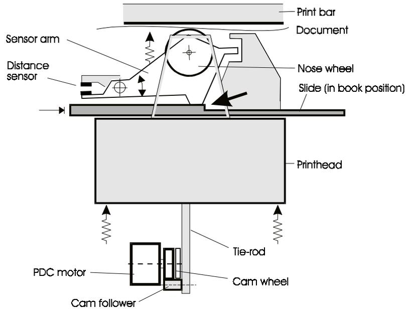
Figure 2-16 Printhead-to-paper mechanism in book position
