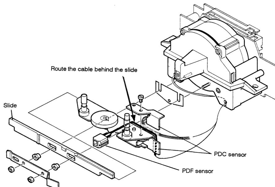
Figure 3-25 Removing the PDF sensor (the sensor can be removed without dismantling the sensor mechanism as shown in this figure)
