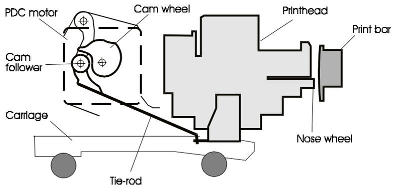
Fig 2-17 Head attach position for passbook printing
