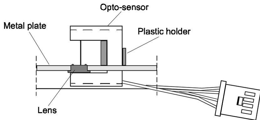
Figure 3-42 Fitting a right edge sensor
