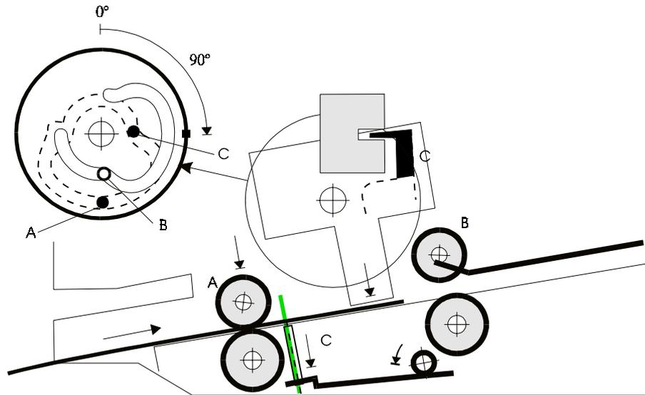
Figure 2-6 The feed motor starting to feed in the document
