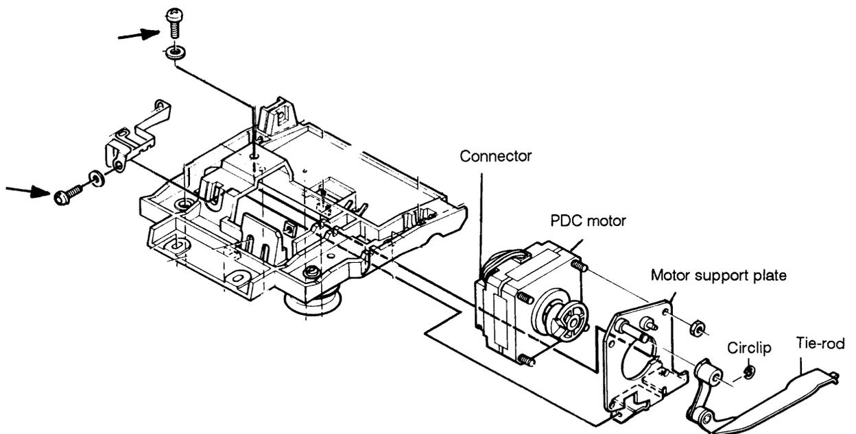
Figure 3-26 Removing the PDC motor (this figure is intended for parts identification only)
