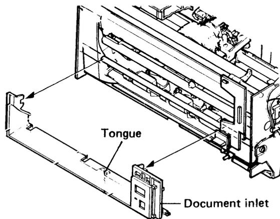
Figure 3-27 Removing the document inlet
