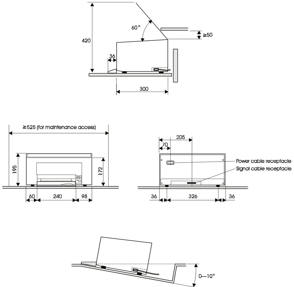
Figure 4-1 Dimensions of the LB12/LB15 printers
