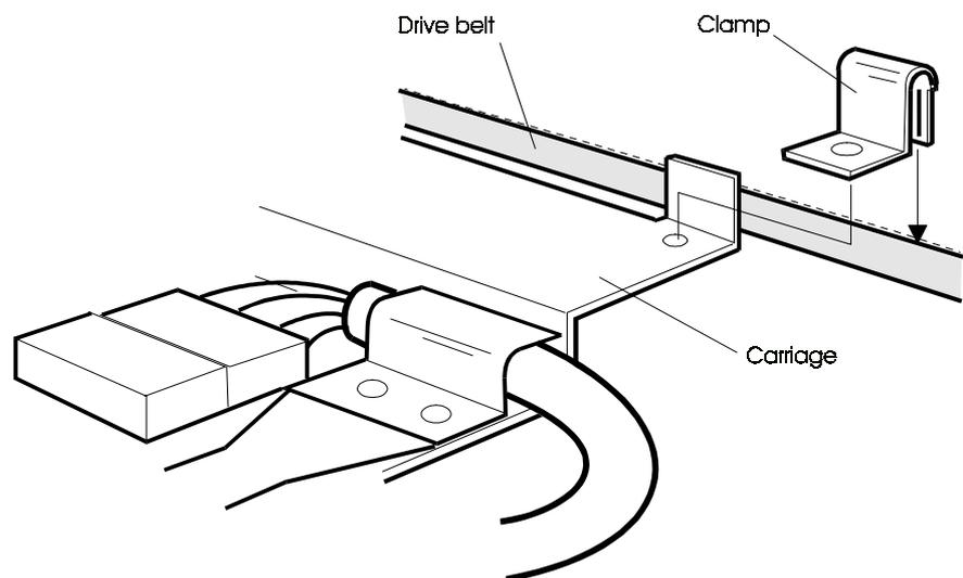
Figure 3-46 Engaging the carriage with the drive belt
