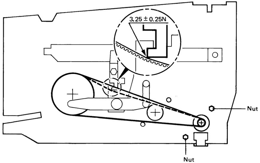
Figure 3-6 Drive belt for the grasp mechanism
