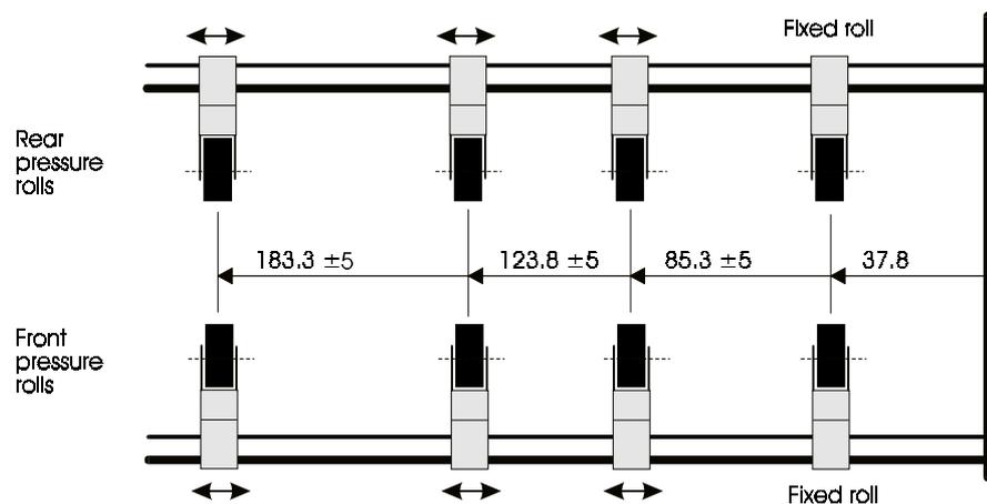
Figure 3-4 Pressure rolls position in the document station
