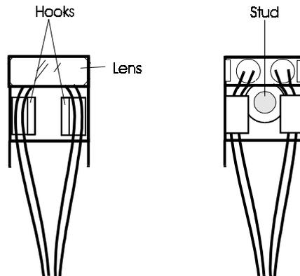
Figure 3-40 Preparing an outer bottom sensor
