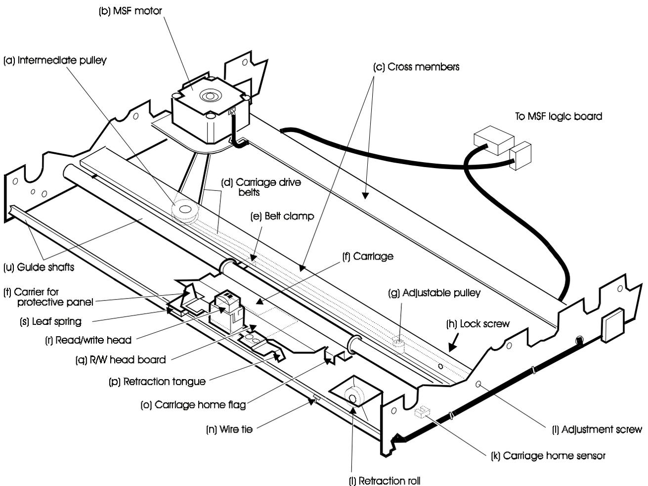
Figure 2-36 MSF mechanics
