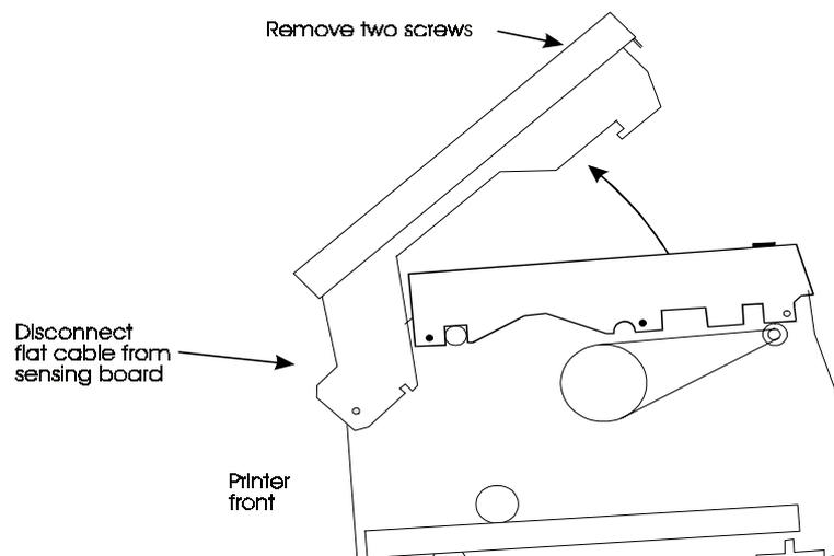
Figure 3-28 Preparing to remove the main board
