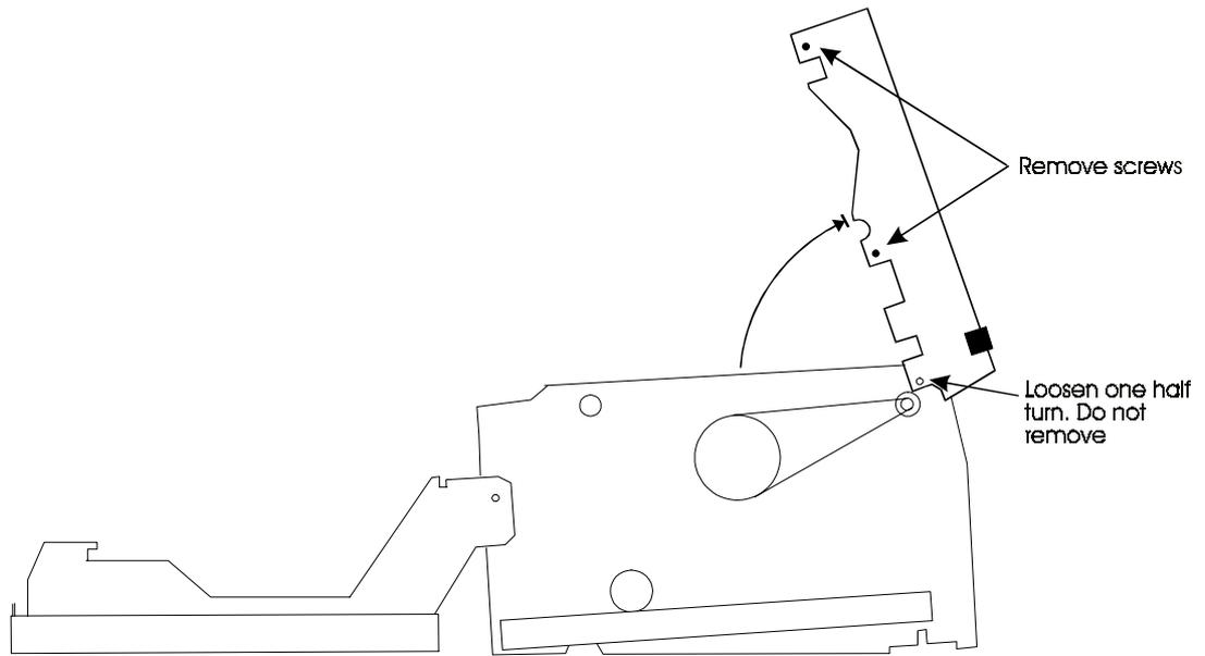
Figure 3-43 Raising the MSF mechanics assembly
