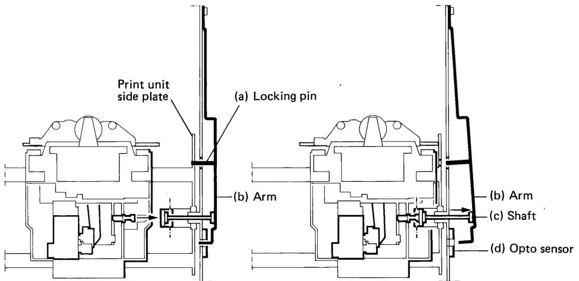
Figure 2-14 Carriage in its extreme right position releases the print unit
