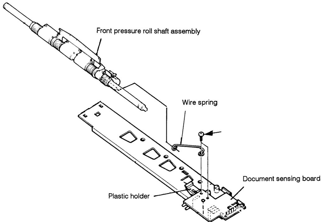
Figure 3-37b Removing the document sensing board (this figure is only intended for parts identification)
