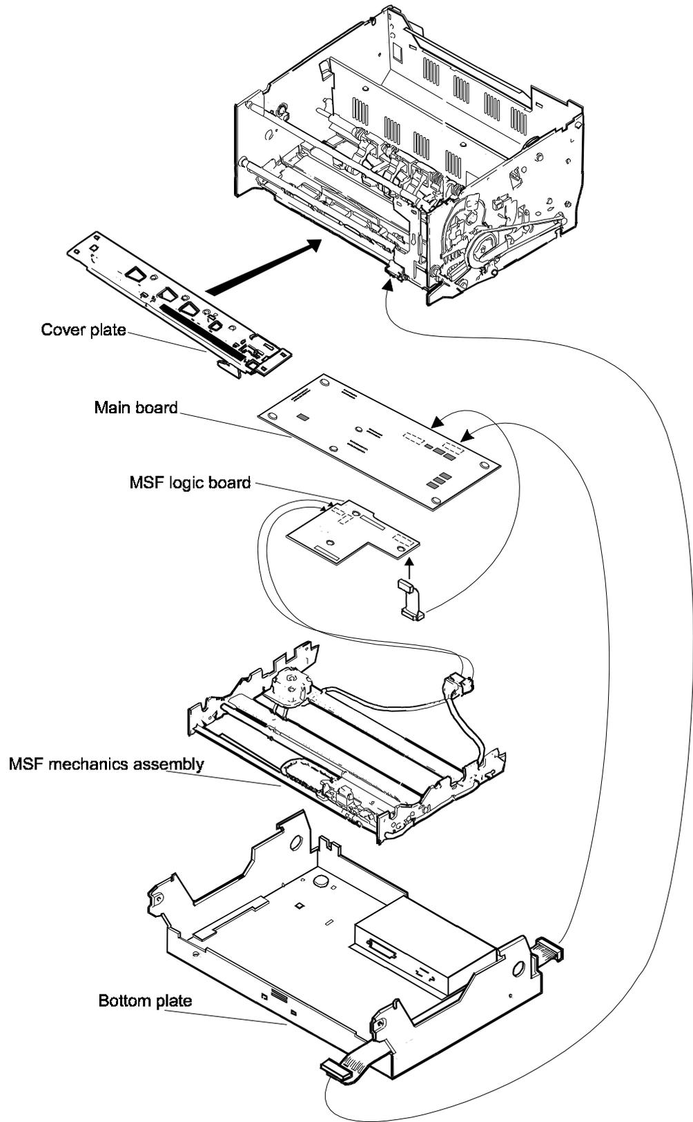
Figure 1-9 The main parts of the MSF device
