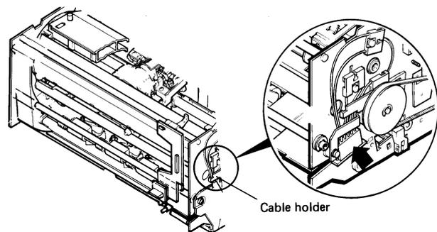
Figure 3-37a Removing the document sensing board
