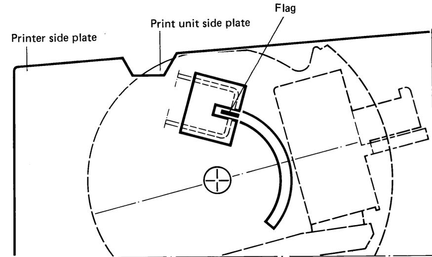
Figure 2-11 Print unit position sensor (V-H sensor)
