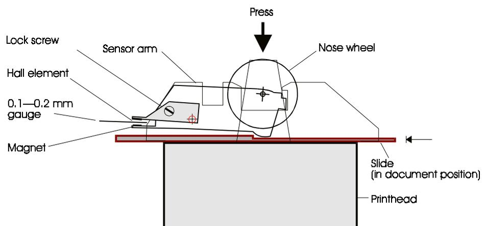
Figure 3-12 Adjusting the PDC sensor gap
