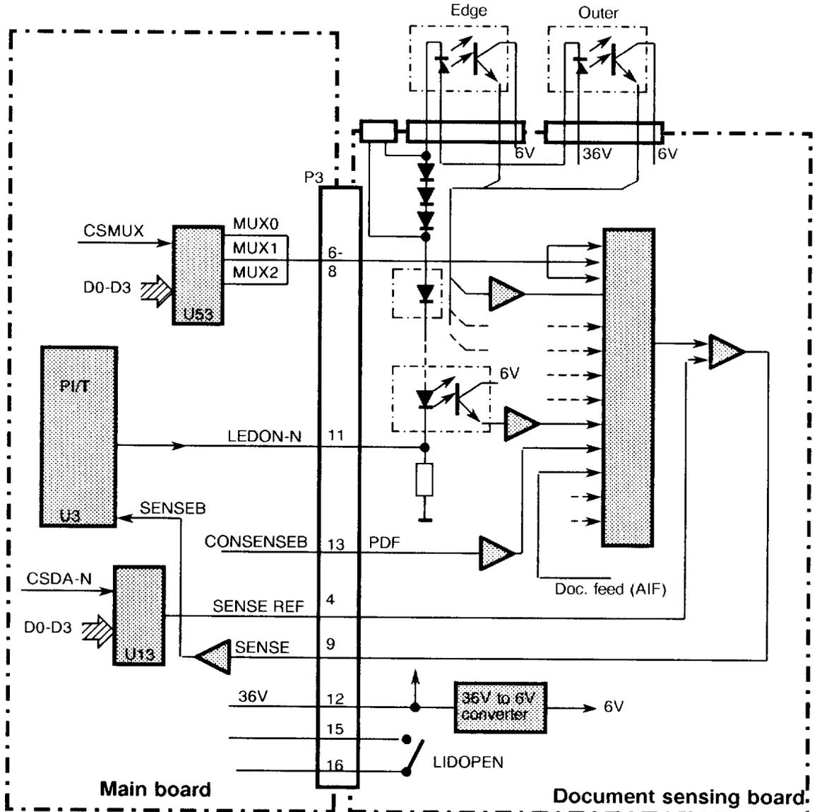
Figure 2-25 Opto-sensor logic
