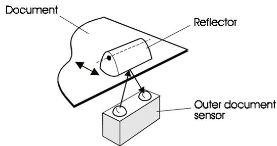
Figure 2-23 Light-reflecting opto-sensor
