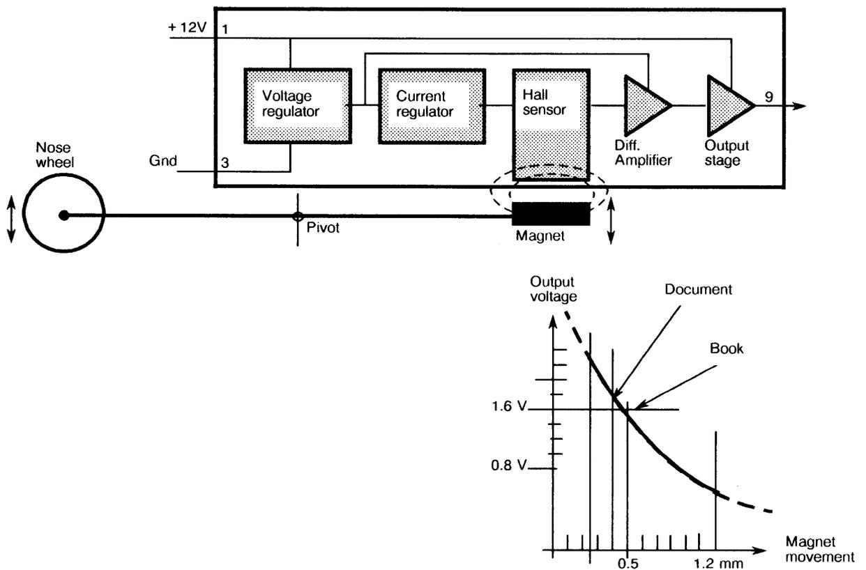
Figure 2-22 PDC sensor element
