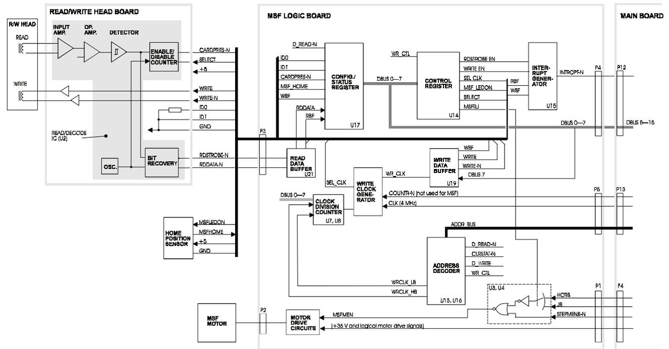
Figure 2-38 MSF block diagram
