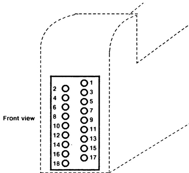
Figure 2-28 Printhead needle arrangement
