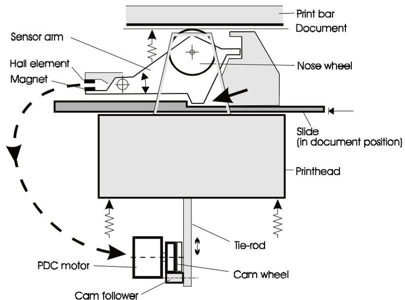
Figure 2-15 Printhead-to-paper distance mechanism in document position
