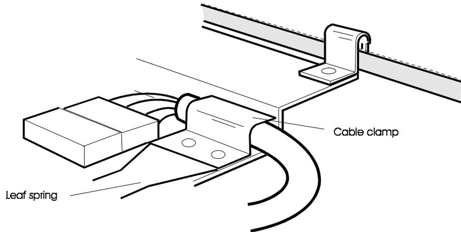
Figure 3-47 Disconnecting the cable from the R/W head board
