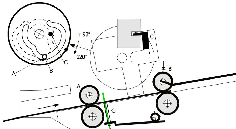
Figure 2-7 Lowering the rear pressure rolls
