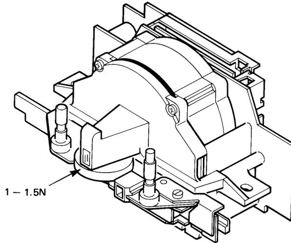
Figure 3-11 Printhead nose wheel
