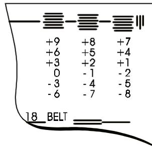
Figure 3-22 Checking the paper feed motor drive belt
