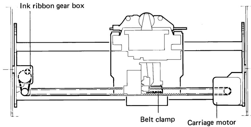
Figure 2-12 Carriage drive mechanism
