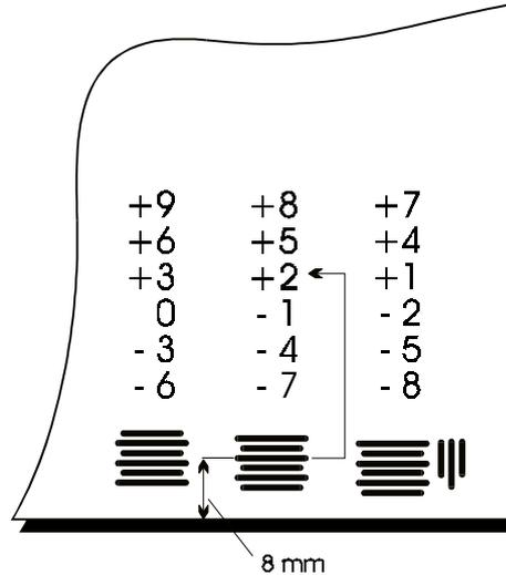
Figure 3-19 Finding the bottom sync offset correction value, example
