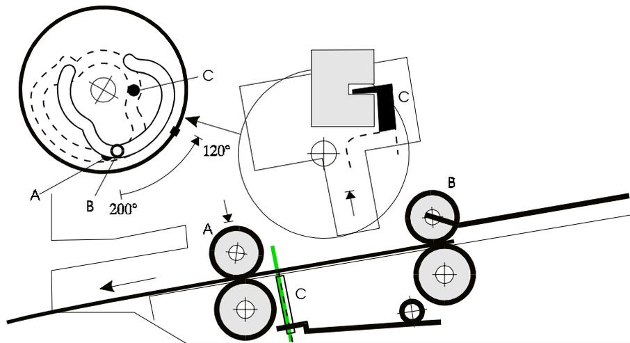
Figure 2-9 Front pressure rolls lowered to complete the document release
