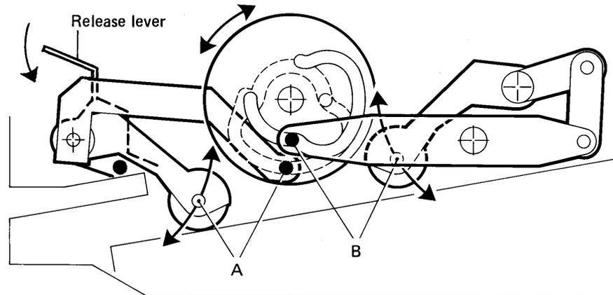
Figure 2-2 Pressure rolls mechanism
