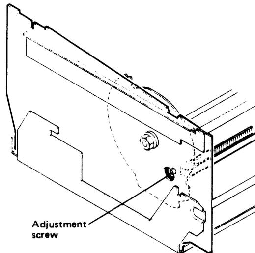
Figure 3-8b Adjusting the carriage drive belt
