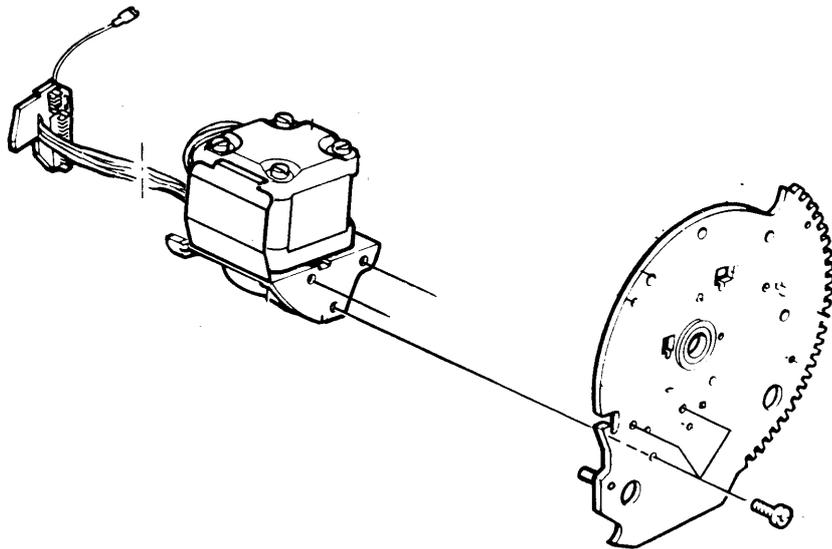
Figure 3-34b Preparing to remove the carriage motor
