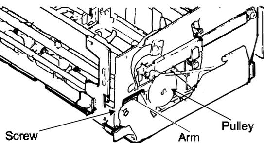
Figure 3-5 Adjusting the front pressure rolls
