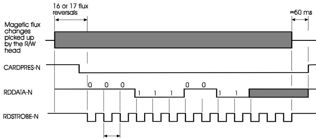
Figure 2-37 Data read signal timing diagram
