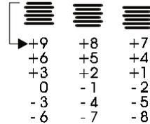
Figure 3-17 Top sync offset graduation lines
