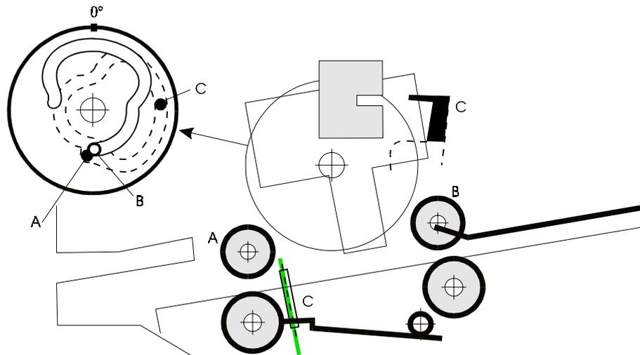
Figure 2-4 Feed rolls and stop pins in home position
