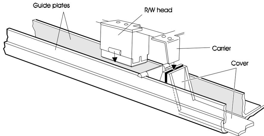
Figure 3-45 Engaging the protective cover carrier
