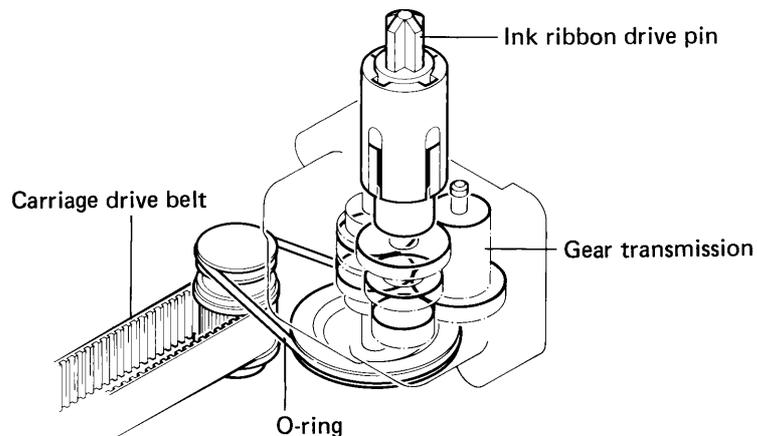
Figure 2-13 Ribbon drive mechanism
