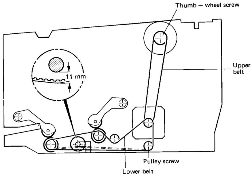
Figure 3-7 Drive belts for the document feed mechanism
