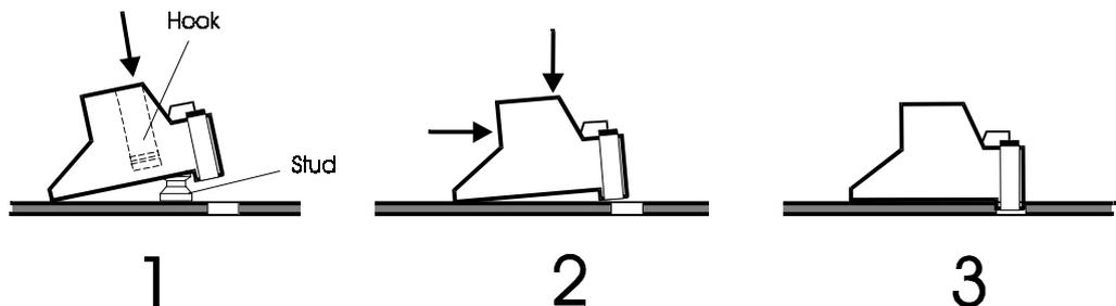
Figure 3-41 Fitting an outer bottom sensor
