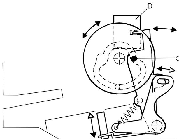
Figure 2-3 Stop pin mechanism
