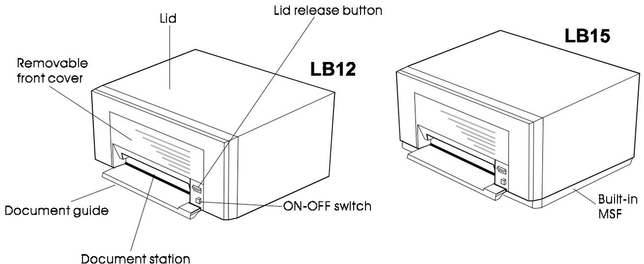
Figure 1-1 The LB12/LB15 printers, exterior
