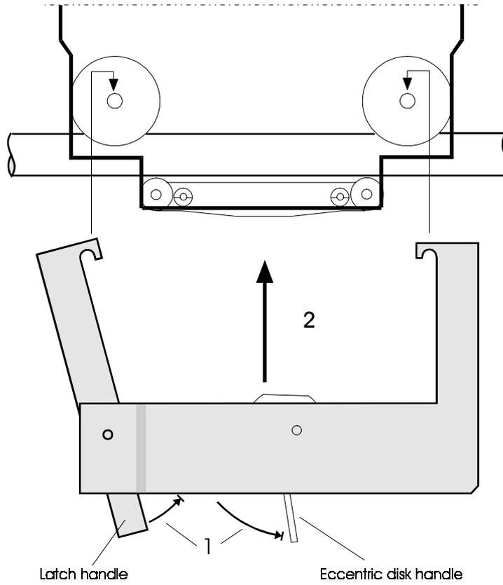
Figure 3-14 Fitting the carriage adjustment tool
