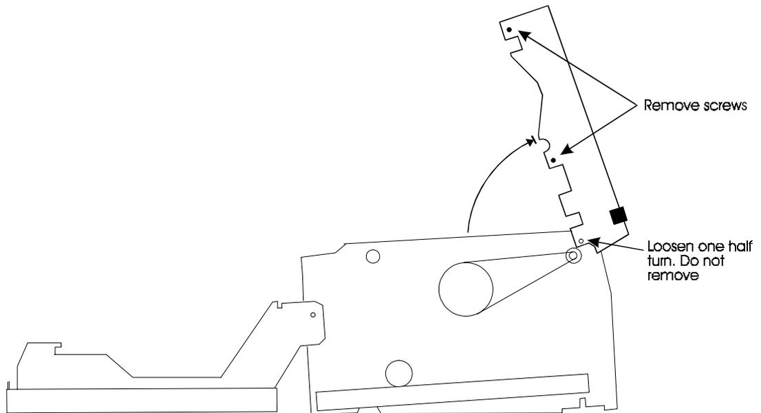
Figure 3-29 Removing the main board
