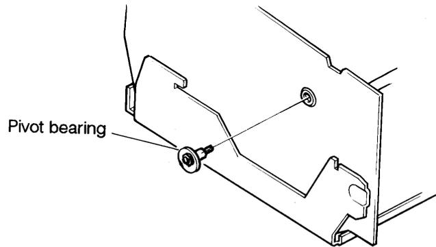
Figure 3-33 Removing the left side pivot bearing
