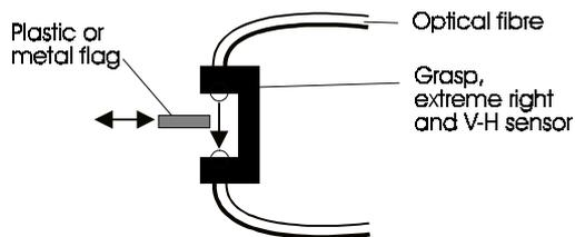
Fig 2-24a Light-breaking opto-sensors
