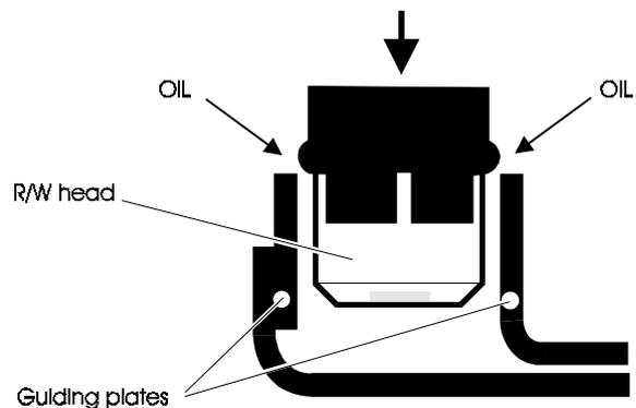
Figure 3-44 Lowering the R/W head between the guide plates
