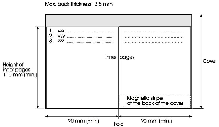
Figure 1-10 Dimensions of vertically folded passbooks
