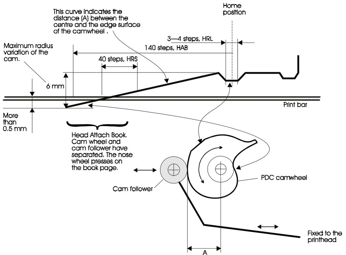
Figure 2-20 The PDC cam wheel
