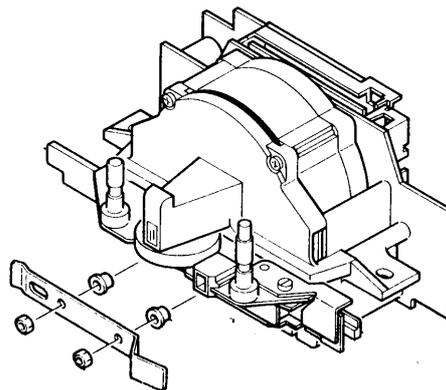
Figure 3-10 Printhead slide (adjustment)
