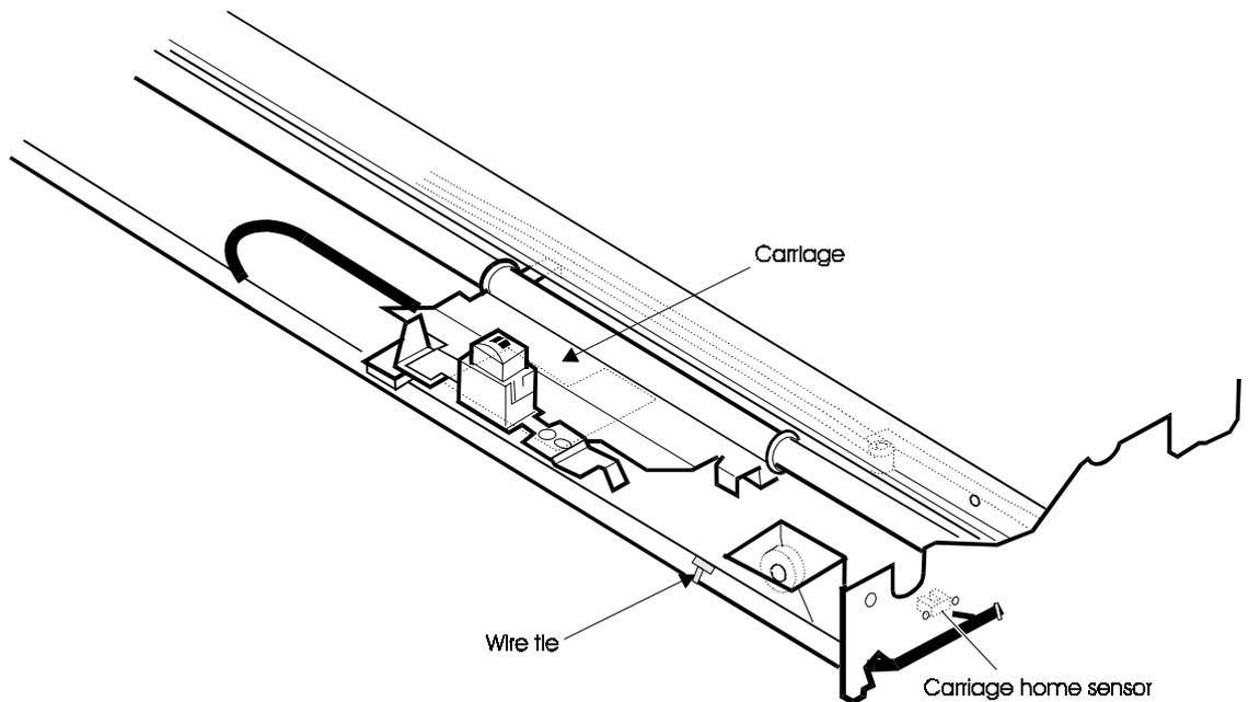
Figure 3-48 Removing the carriage home sensor
