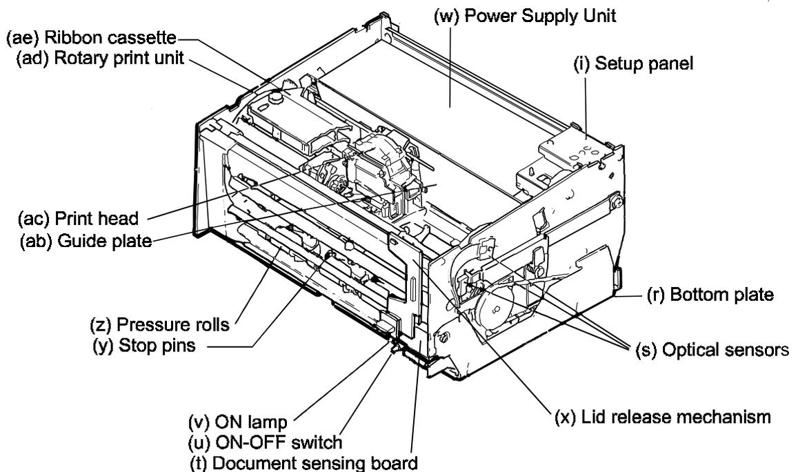
Figure 1-3 Printer modules
