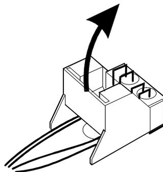
Figure 3-39 Removing an outer bottom sensor
