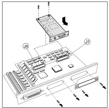
PLUG THE APPLETALK INTERFACE CONNECTOR INTO LOCATION J7 OR J9 AND SECURE.
