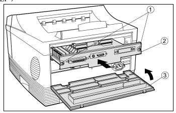
REINSTALL AND SECURE THE CONTROLLER BOARD AND CLOSE THE REAR COVER.
