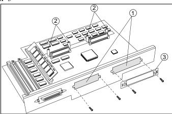
REMOVE THE BLANK PLATE COVERING EITHER INTERFACE CONNECTOR SLOT.
