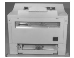
3. Press the tabs at the left and right of the panel and drop the panel down.
