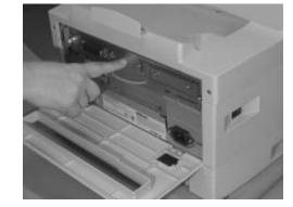
5. Unscrew the captive screws at the left and right of the assembly.
