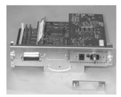
6. Slide the assembly into the printer. Press firmly and evenly on each side of the assembly to seat it.
