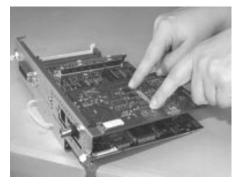
5. Use the screws supplied with the NIC to attach the face plate to the option port.
