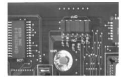
3. To enable the LAT protocol, move Jumper 8 to the ON position.
