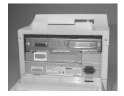
4. Touch the metal chassis to discharge static electricity.
