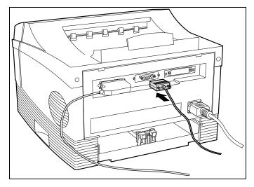
ATTACH ONE END OF THE SERIAL CABLE TO THE PRINTER AND ATTACH THE OTHER END TO THE SERVER OR HOST COMPUTER.
