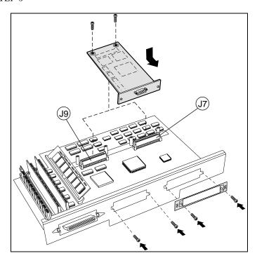
PLUG THE SERIAL BOARD INTERFACE CONNECTOR INTO LOCATION J7 OR J9 AND SECURE.
