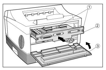
REINSTALL AND SECURE THE CONTROLLER BOARD AND CLOSE THE REAR COVER.
