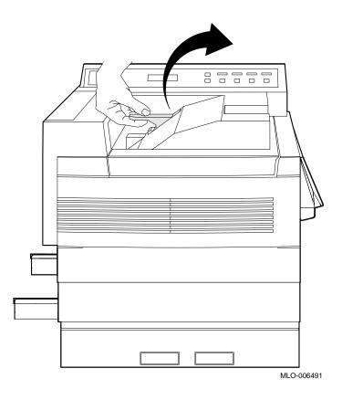
2. Rotate the adjustment knob clockwise to make the print darker, or counter-clockwise to make the print lighter.
