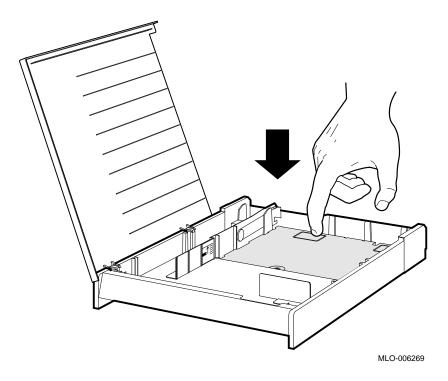
5. Tap a stack of paper on a flat surface to align the edges.
