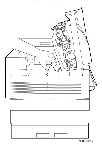
3. Open the left side cover and lift the tab on the fusing unit gate to remove any jammed paper.
