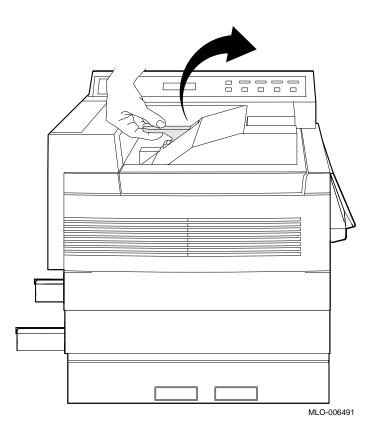
3. Grasp each (green) end of the transfer/separation charger and lift it out of the printer.
