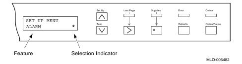
Figure 3-5 shows an example of feature information displayed when the printer is in Menu Mode.
