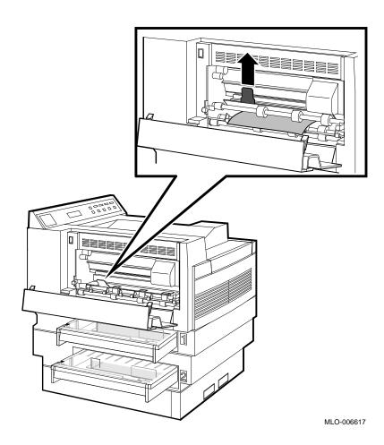
4. Close the fusing unit gate back to its operating position and close the left side cover.
