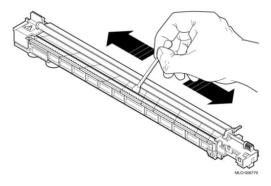
6. Hold the charger upright in the vertical position and clean the toner from the sawtooth comb with the cleaning brush.
