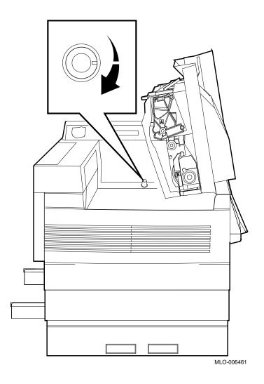
3. Close the top cover by pushing it down until it latches securely in place.
