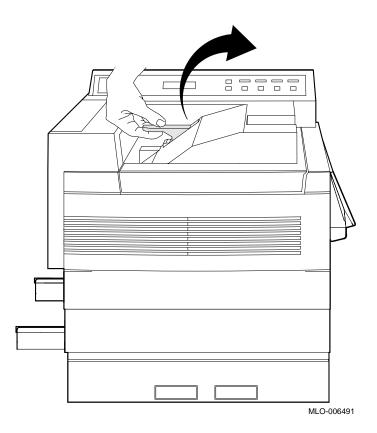
2. Remove any jammed paper inside the printer.
