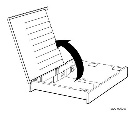
4. Press down the lifting plate to lock it in the loading (lowered) position.
