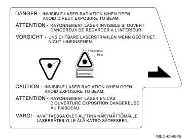
**NOTE:** This label is attached to the laser scanner unit inside the printer.
