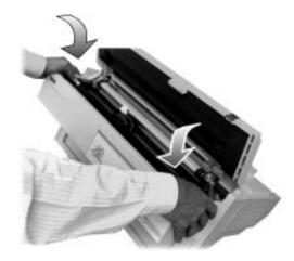
7. Push the cartridge down with your finger over the mounting pins.
