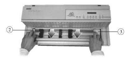
Removing the Tractor Unit
