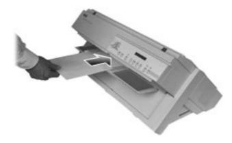
Inserting the Cut Sheet
