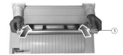
5. Push the Push tractor unit 3 into the printer on both sides until it engages.
