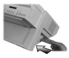
Inserting the Set-Up Card
