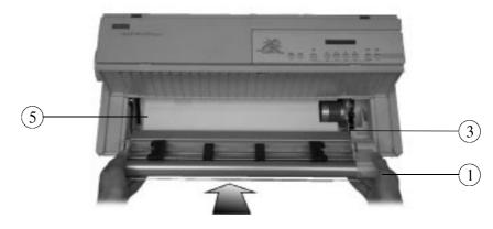
4. Identify the place (5) of the Push tractor unit (1) in the printer. The electrical connector (3) must be on the right.
