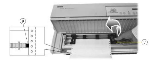
Aligning the Paper Edge with the Green Mark
