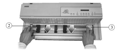
Removing the Tractor Unit
