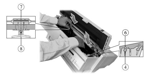
Positioning Cartridge/Aligning Ribbon Guide with Print Head
