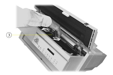
Checking the Ribbon Cartridge Installation
