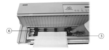
Positioning the Right Tractor/Placing the Paper
