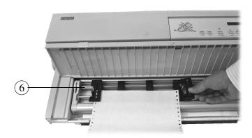
Positioning the Right Tractor/Placing the Paper
