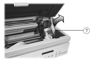
Removing the Carriage Motor Shipment Lock
