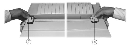
Inserting the Left Cut-out Pull Tractor Pins Cover
