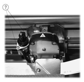
Fixing the Color Mechanism on the Carriage Assembly
