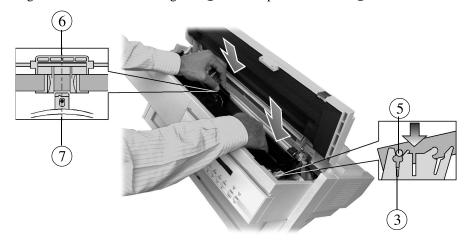
Positioning Cartridge/Aligning Ribbon Guide with Print Head
