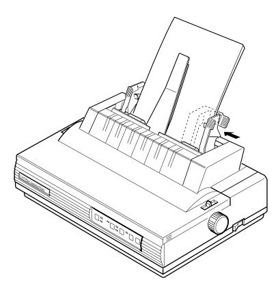
**3** Push the rear tabs on both paper guides towards the back of the printer to secure the paper against the guide rollers.
