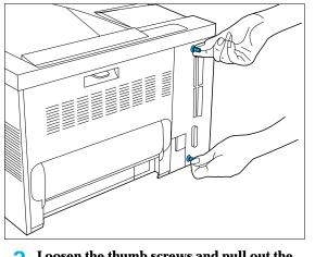
2 Loosen the thumb screws and pull out the controller board.
