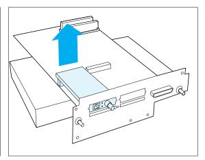
**5** Gently lift up on the card until it detaches from the controller board.
