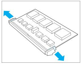
**4** Carefully pull out on the locking clips to release the PostScript SIMM.
