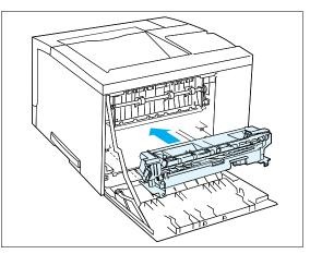
7 Slide the new fuser cartridge into the printer.
