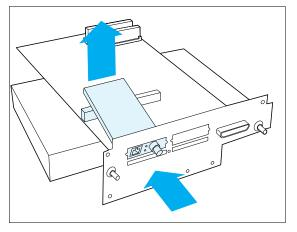
**6** Lift the card out and away from the slot in the controller board. Then replace the screws and faceplate that came with the printer.
