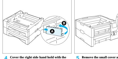
joint tab, inserting (A) then (B).
