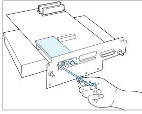
**4** Unscrew the DNIC mounting bracket from the controller board.
