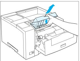
2 Remove the old EP cartridge by lifting it towards the rear of the printer then pulling it up and out.
