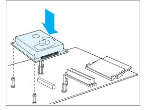
**4** Align the hard drive connector to the controller connector (J180), and gently lay the hard drive on top of the four standoffs.
