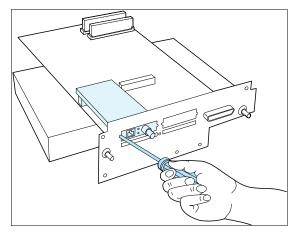
7 Secure the DNIC mounting bracket to the controller board with the screws removed in Step 4.
