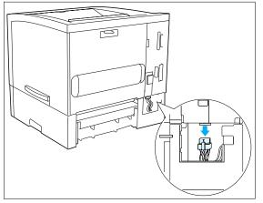
**2** Remove the small cover at the back of the Paper Deck, then unplug the connector from the printer. Replace the small cover.
