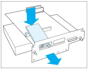
**5** Line up the DNIC connector to the slot in the controller board.
