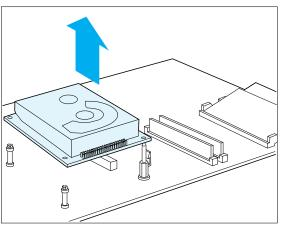
**5** Gently release the opposite end of the hard drive from the standoffs, then lift the hard drive from the controller board.
