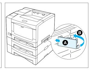
Cover the right side hand hold with the 7 joint tab, inserting (A) then (B).
