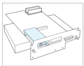
**3** Place the controller board on a ream of paper.
