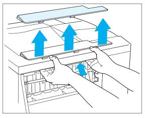
**3** Remove the option interface cover by pushing up on it from the underside. Then close the rear cover.
