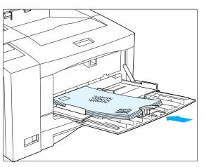
6 When feeding envelopes, slide the end of the envelope stopper over the end of the envelope stack.
