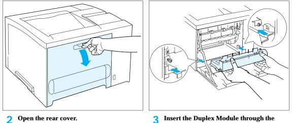
Insert the Duplex Module through the 3 guide channels.
