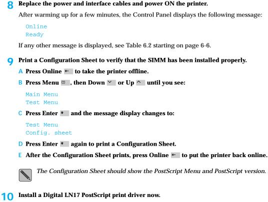
Table 2 in the *Setting Up Guide* lists the LN17 PostScript printer drivers packaged with your printer. See the *Setting Up Guide* for installing driving software.
