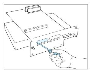
**4** Place the controller board on a ream of paper and remove the screws and faceplate from the slot where you will install the DNIC.
