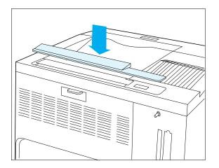
4 Replace the option interface cover which was removed and stored when the option was first installed.
