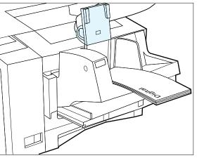
**1** Lift the envelope holder and stack the envelopes in the feeder.
