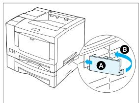
**3** Cover the right side hand hold with the joint tab, inserting (A) then (B).
