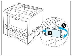
4 Remove the right joint tab joining the printer to the Paper Deck, removing (A) then (B).
