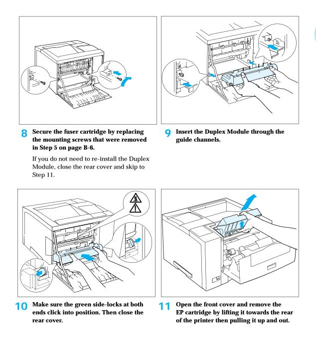
Replacing the Fuser Cartridge/BTR
