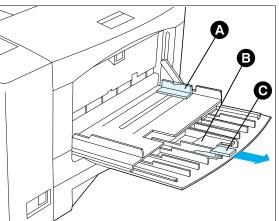
2 Slide the side guide (A) to the far right. Flip open the extension bar (B) if feeding long paper. Pull out the envelope stopper (C) if feeding envelopes.
