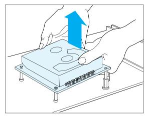
**4** Gently unlatch the hard drive from the standoffs and release the hard drive connector from the controller board connector.
