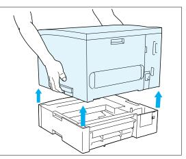
**5** Holding the printer by the recessed side hand holds, lift it up off the Paper Deck.
