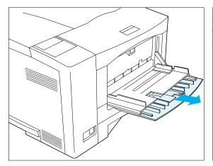
**1** Press the top of the front tray to open it, then pull out the tray extension.
