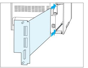
8 Replace the controller board, sliding it along the alignment channels. Then hand-tighten the thumb screws.
