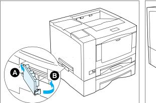
**4** Cover the left side hand hold with the joint tab, inserting (A) then (B).
