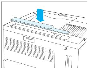
3 Replace the option interface cover which was removed and stored when the option was first installed.
