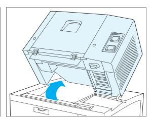
**3** Carefully lift the Mailbox/Collator off the printer, rotating it away from the rear of the printer.
