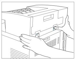
2 Press the release buttons with your thumbs and push up on the OCT to remove it.
