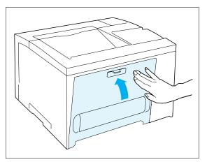
**5** Close the rear cover, plug in the power cord, and power ON the printer.
