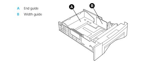
The end guide (A) slides to fit the length of the paper.
