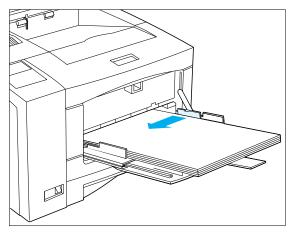
5 Adjust the side guide to the size of the paper loaded in the front tray.
