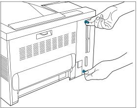
**3** Loosen the thumb screws and pull out the controller board.
