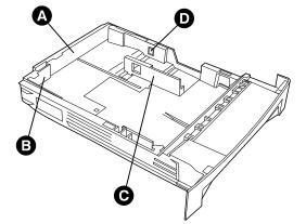
Figure 2.2 Main tray paper adjustment guides
