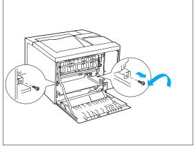
5 Remove the mounting screws from the printer as shown above, and set them aside.
