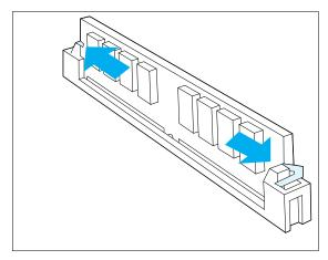
**4** Carefully push out on the locking clips to release the SIMM.
