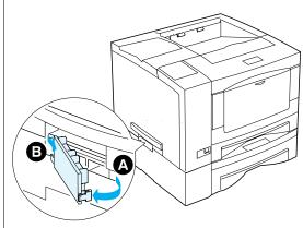
**3** Remove the left joint tab joining the printer to the Paper Deck, removing (A) then (B).
