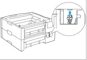
Remove the small cover at the back of the 5 bottom Paper Deck. Fit the connector firmly into the top Paper Deck receptacle. **Replace the small cover.**
