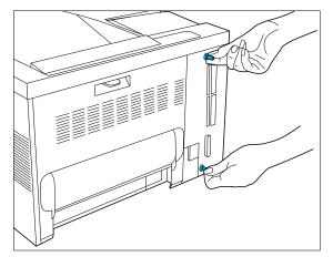
2 Loosen the thumb screws and pull out the controller board.
