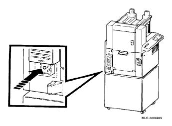
2. Connect one end of the power cord to the AC input power receptacle at the rear of the printer.
