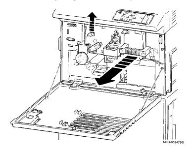
3. Open the cover of the development unit by lifting the right side of the cover up and over to the left side of the development unit.
