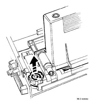
8. Attach knob to the take-up roller and turn the knob clockwise until the red line appears on the take-up roller.
