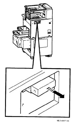
3. Reinstall the two thumbscrews to secure the Ethernet connector in the operating position.
