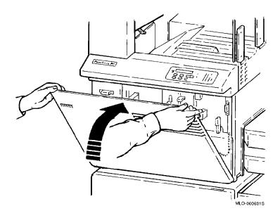
8. Open the cabinet door and remove the tape from the duplex transport guide and the transfer/separation charger cleaner. Remove the carton containing two toner cartridges from the cabinet.
