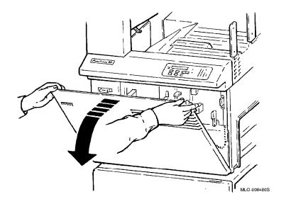
2. Open the development drawer by lifting up the development drawer release lever while pulling the drawer out by its handle until it stops.
