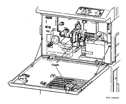
4. Open the development drawer by lifting up the release lever while pulling the drawer out by its handle until it stops.
