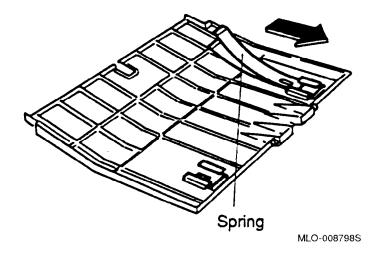
3. Install a paper tray insert into the lower output tray.
