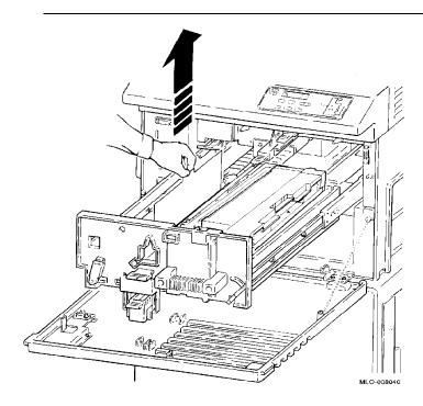
6. Push the development unit release lever back to the operating position.
