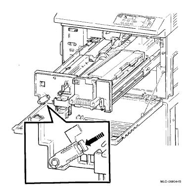
2. Turn the development unit release lever clockwise to disengage the development unit from its operating position.
