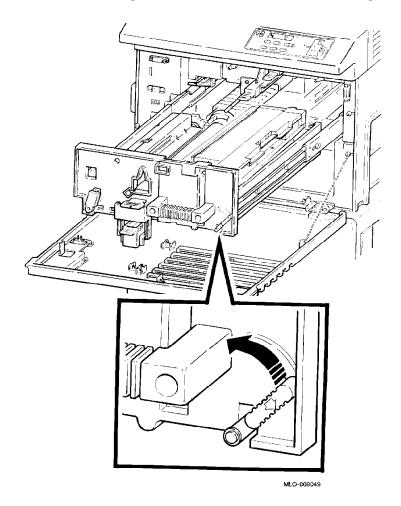
7. Push the cleaning unit release lever back to the operating position.
