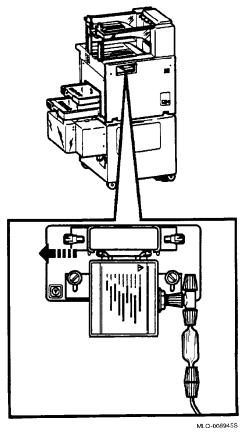
4. Raise the bracket until it touches the DESTA and tighten the two thumbscrews.
