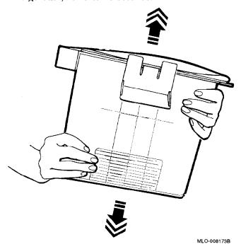
5. Install the right side of the cartridge into the hinges of the frame.
