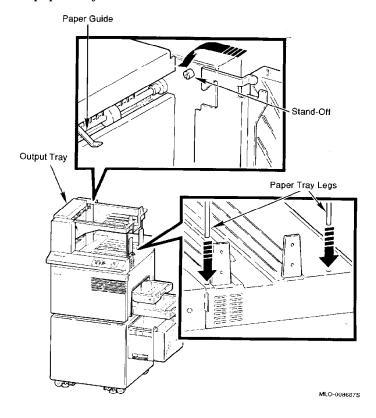
3. Install a paper tray insert into the top output tray.
