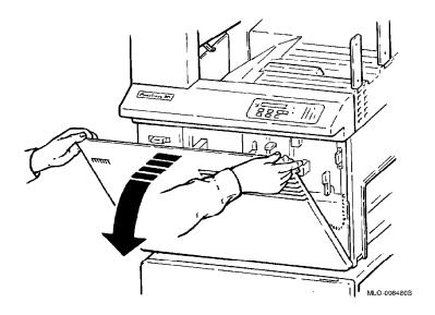
3. Remove the tape and foam padding from the print engine. Also, remove the one piece of tape and foam padding from the print engine cover.
