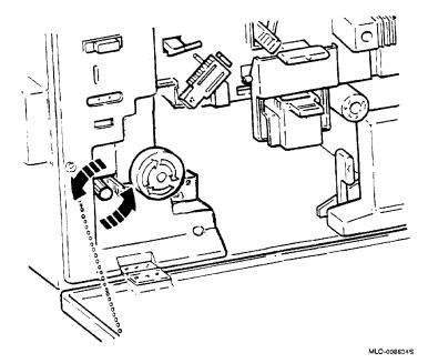
$3. \;\;$  Push the lever to the left. Pull out the fusing unit until it stops.
