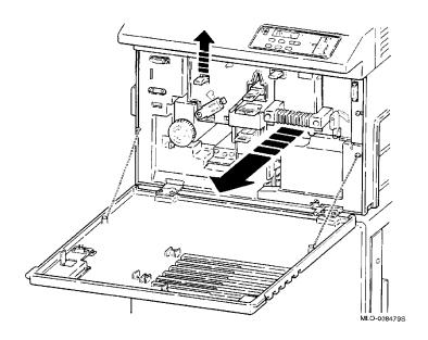
3. Make sure the cleaning unit, OPC drum, and toner cartridge are seated correctly.
