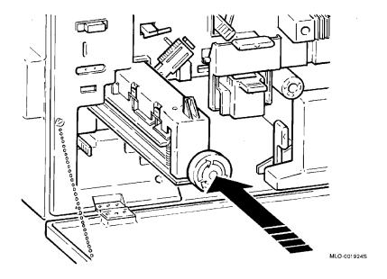
5. Replace the screw next to the fusing unit release lever.
