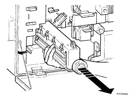
4. Push the fusing unit in until it is firmly seated in the printer.
