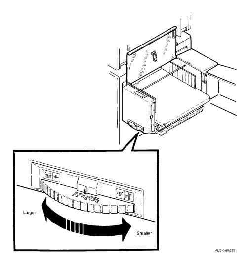
3. Install the base plate, being sure the bottom paper tray pins come up through the plate holes and the plate hooks in place. Make sure the size of the base plate matches the size indicated on the paper size dial.
