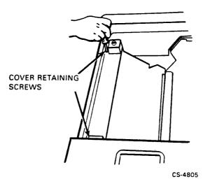
Figure 4-4 Cover Retaining Screws
