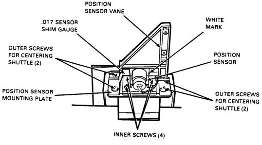
Figure 4-41 Position Sensor Gap Adjustment
