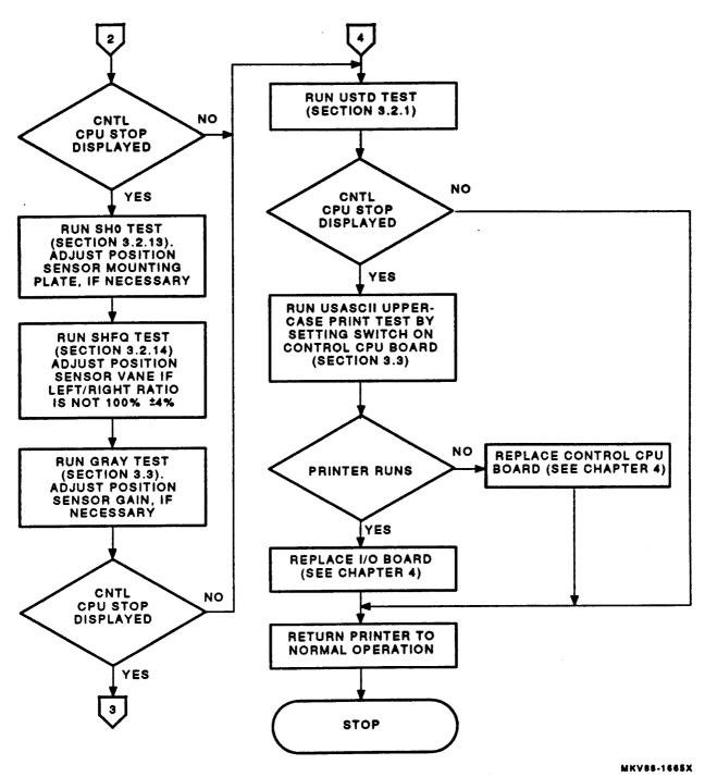
Figure 2-1 CNTL CPU STOP Flowchart (Sheet 3 of 3)
