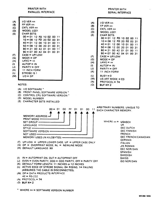
Figure 3-11 Configuration Test (Serial and Parallel I/O) Printout
