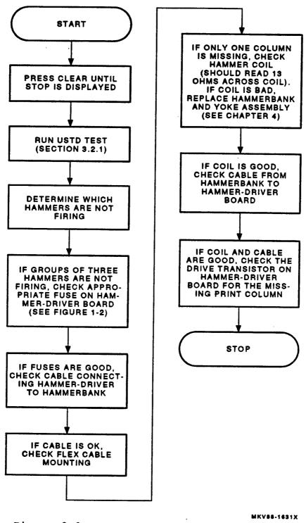
Figure 2-2 ERRE HAMMER FAULT Flowchart
