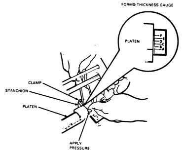
Figure 4-28 Right Platen Clamp and Forms-Thickness Gauge
