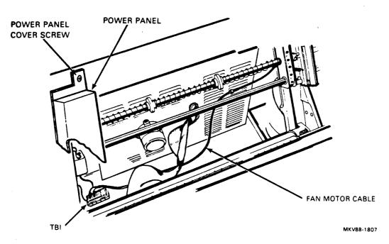
Figure 4-46 Blower Motor Cable Leads
