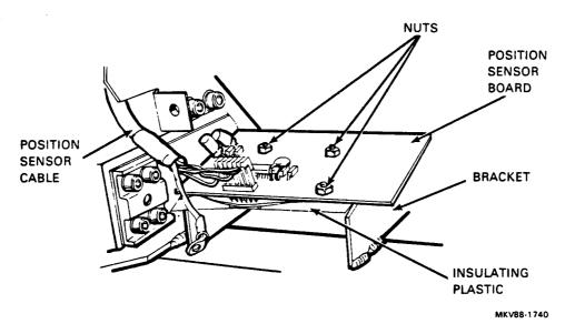
Figure 4-54 Shuttle Position Sensor Board
