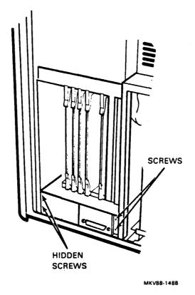
Figure 4-60 Bulkhead Panel Assembly
