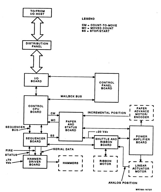
Figure 1-4 LG01 Electronics Block Diagram
