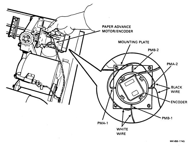
Figure 4-47 Paper Advance Motor/Encoder Location
