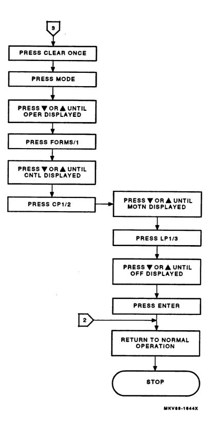
Figure 2-11 PAPM MOTION Flowchart (Sheet 3 of 3)
