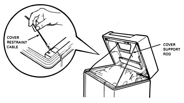
Figure 4-5 Cover Support Rod and Cover Restraint Cable
