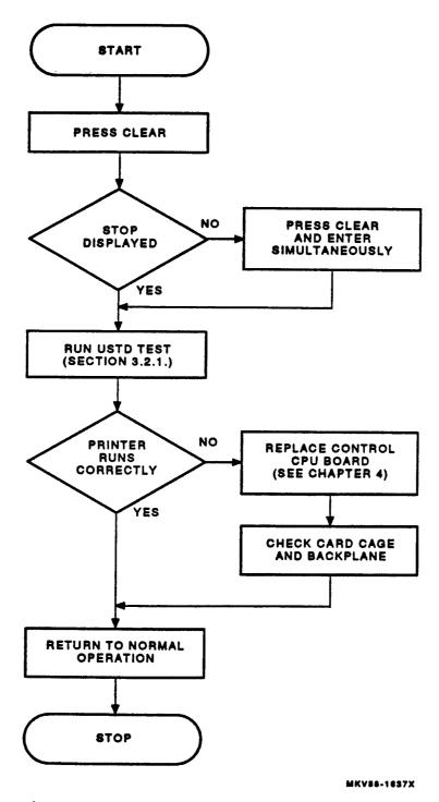
Figure 2-6 ERR6 ELEC FAULT Flowchart
