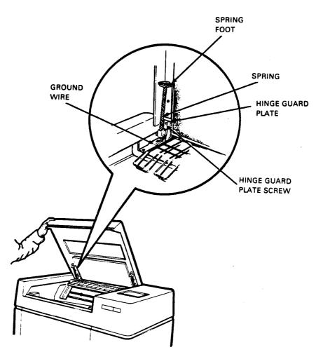
Figure 4-3 Lid Hinge Springs and Hinge Guard Plate
