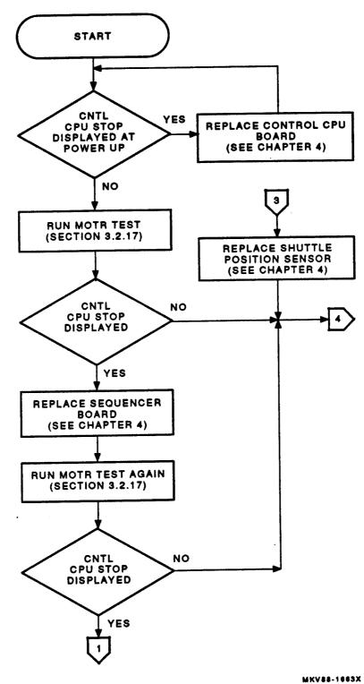
Figure 2-1 CNTL CPU STOP Flowchart (Sheet 1 of 3)
