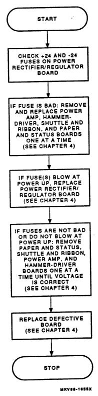
Figure 2-18 +15 VOLT POWER or -15 VOLT POWER Flowchart
