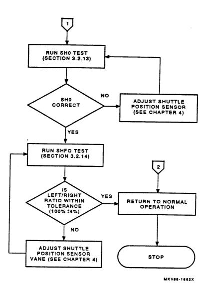
Figure 2-22 Varying Gap Between Characters Flowchart (Sheet 2 of 2)
