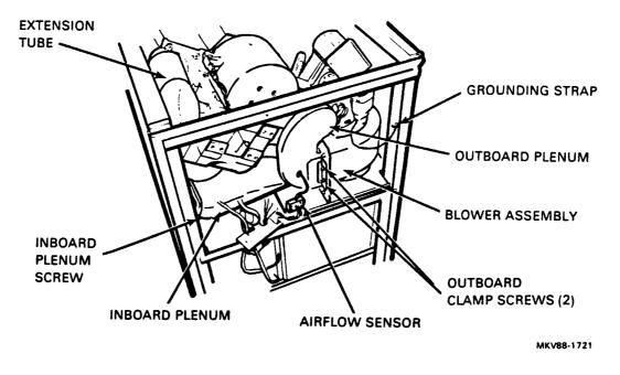
Figure 4-24 Air System Components
