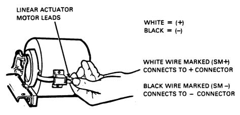
Figure 4-50 Linear Actuator Motor Leads
