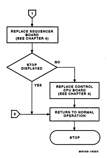
Figure 2-4 ERR3 SEQ RAM Flowchart (Sheet 2 of 2)
