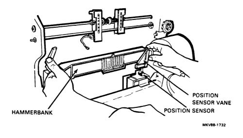
Figure 4-38 Hammerbank Removal
