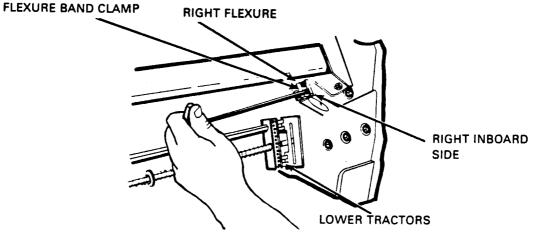
Figure 4-37 Lower Flexure Band Clamp Location
