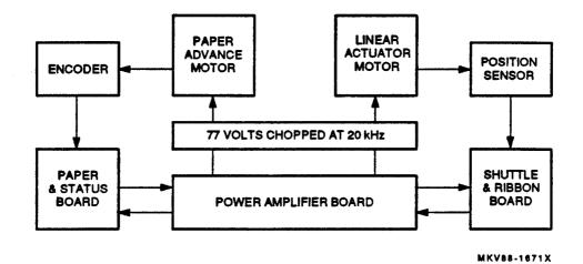
Figure 1-10 Power Amplifier Board Block Diagram
