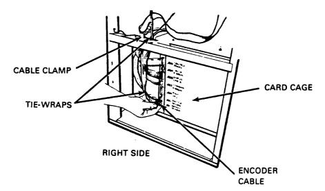
Figure 4-48 Encoder Cable and Card Cage Connection
