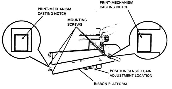
Figure 4-31 Ribbon Cartridge Support Assembly and Ribbon Platform
