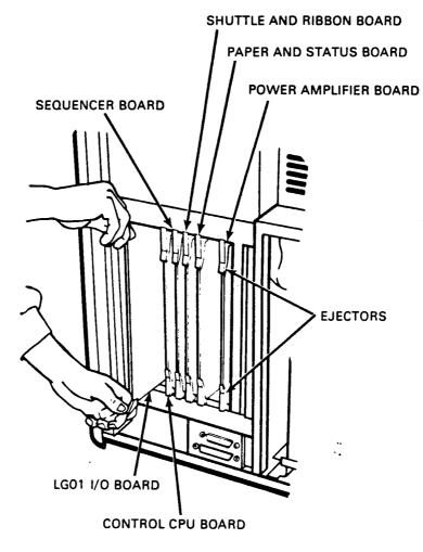
Figure 4-12 Card Cage Boards and Ejectors
