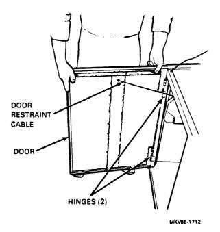
Figure 4-8 Front Door Removal
