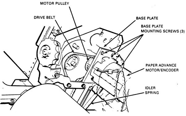
Figure 4-49 Paper Advance Motor/Encoder Components
