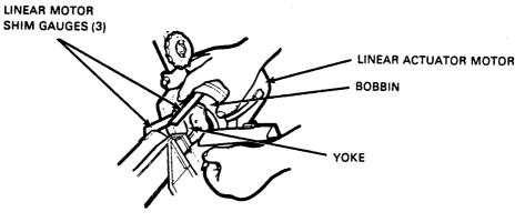
Figure 4-33 Linear Motor Shim Gauges
