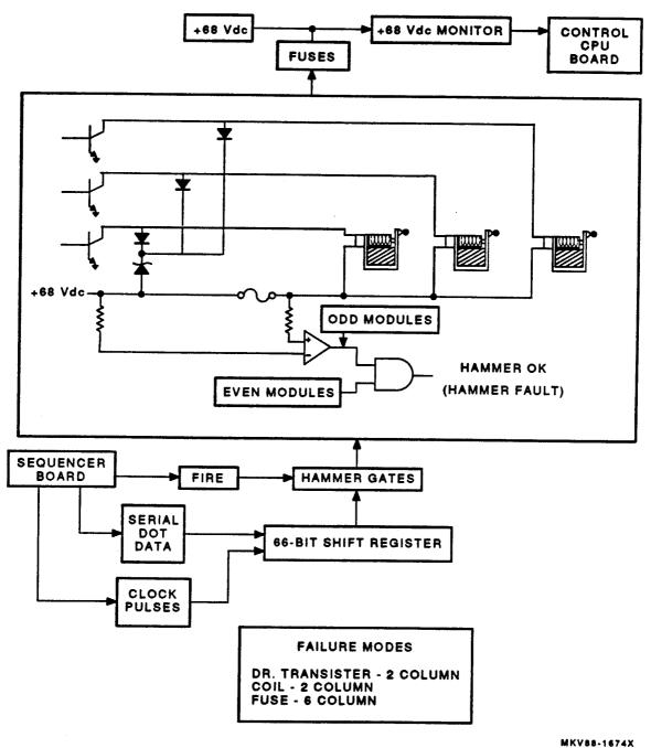
Figure 1-11 Hammer-Driver Board Block Diagram
