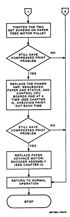
Figure 2-21 Compressed Print Flowchart (Sheet 2 of 2)
