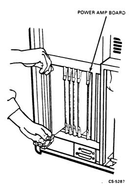
Figure 4-55 Power Amplifier Board Removal
