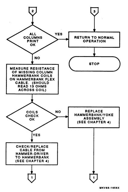
Figure 2-20 Missing Print Flowchart (Sheet 2 of 2)
