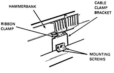
Figure 4-35 Hammerbank Cable Clamp Bracket
