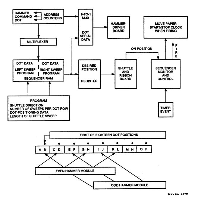
Figure 1-7 Sequencer Board Block Diagram
