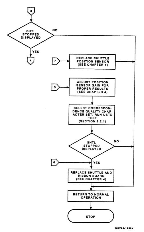
Figure 2-14 SHTL STOPPED Flowchart (Sheet 3 of 3)
