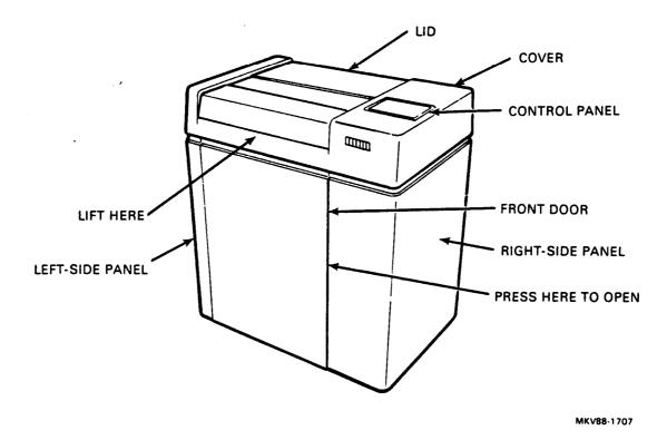
Figure 4-1 LG01 Line Printer Outer Covers
