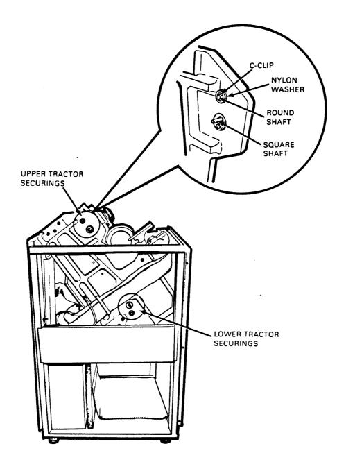
NOTE THIS DETAIL SHOWS THE UPPER TRACTOR SECURINGS. THE LOWER TRACTOR SECURINGS ARE REVERSED IN POSITION (ROUND SHAFT ON THE BOTTOM).
