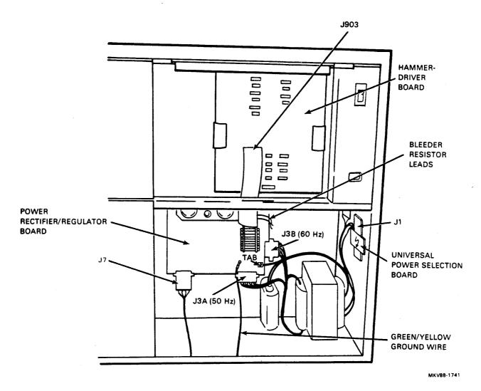
Figure 4-57 Location of Power Supply Components
