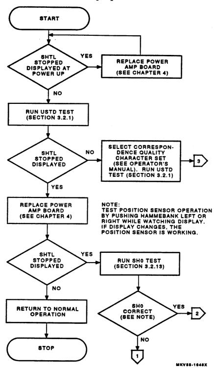
Figure 2-14 SHTL STOPPED Flowchart (Sheet 1 of 3)
