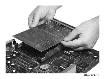
9. Install the new Twisted-pair daughter board by aligning the holes over the retaining clips.
