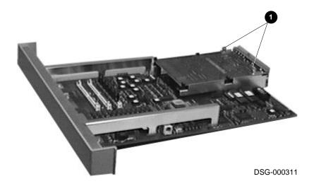
7. Spread the four retaining clips  $\ensuremath{\mathbf{0}}$  to release the daughter board.
