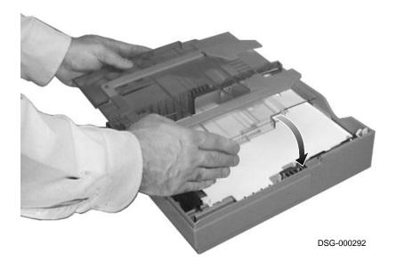
5. Remove the evelope feeder slot cover by sliding it straight down.  $\surd$  Store the cover for future use.
