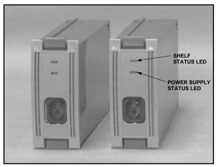
Figure 1-2 Power Supply LEDs
