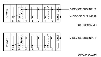
Each bus requires a terminator. The terminator (T) and jumper (J) connectors are mounted on the rear of the backplane.
