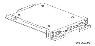
You can remove and install an EMU without removing power, shutting down the controller, or quiescing the SCSI bus.
