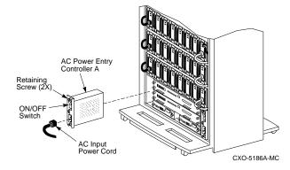
4. Remove the power controller from the enclosure and place it in an electrostatic bag.
