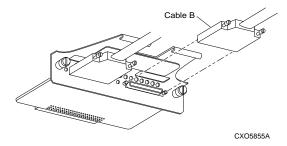
Gently insert the cable connector into module connector. Tighten both cable connector thumb screws to fully seat the connector.
