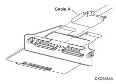
Gently insert the cable connector into module connector. Tighten both cable connector thumb screws to fully seat the connector.
