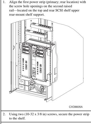
3. Repeat steps 1 and 2 for the second power strip (redundant; front location) using the front raised rail on the upper rear-mount shelf support.
