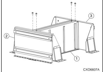
3. Turn the three bracket assembly over (upside-down), exposing the face of shelf.
