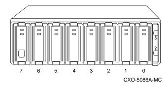
Figure 5-14 BA356 Shelf with 8-Bit I/O Module
