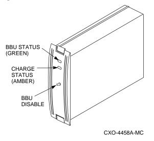
These LEDs are controlled by internal BBU signals. The BBU status LED has three states: on, off, and flashing. The charge status LED is either on or off. **Error! Reference source not found.** defines the valid states for these LEDs.
