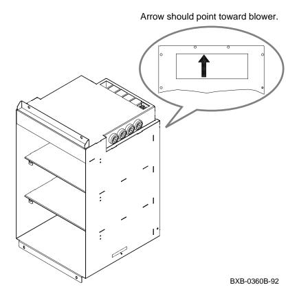
The arrow on the rear panel of the PIU enclosure must point toward the blower. That is, the arrow must point up when installing the PIU below the blower; it must point down when installing the PIU above the blower.
