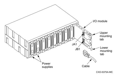
Figure 4-3 Controller Shelf with I/O Connectors
