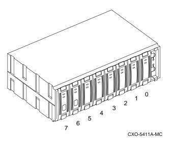
Figure 2-2 SBB Shelf with I/O Module
