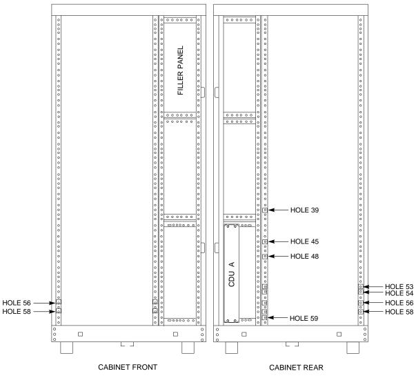
Figure 3–3 Install U-Nuts on Cabinet Vertical Rails
