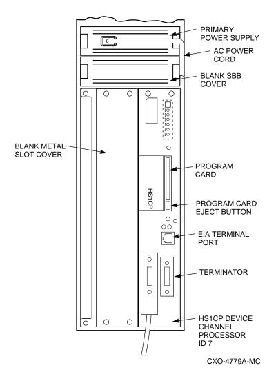
6. Install the blank SBB cover over the open lower power supply slot (see Figure 3–17).
