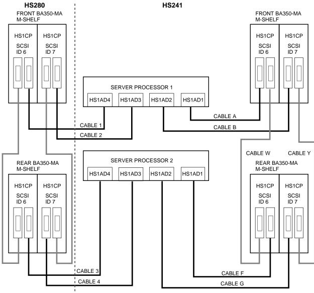
Figure 9–8 Cabling Diagram for HS241/HS280
