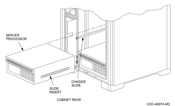
When installed, the server processor should be able to move in both directions.
