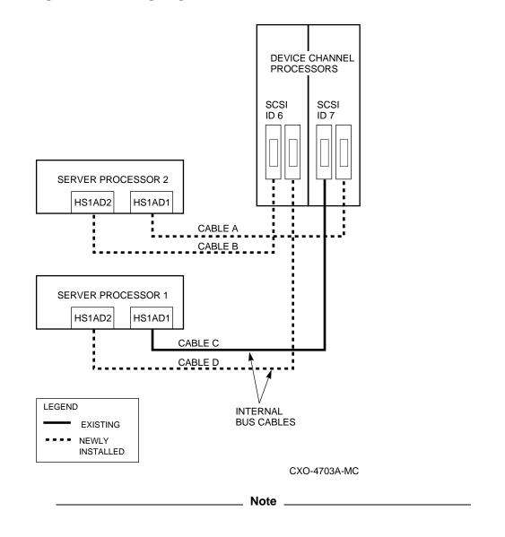
Figure 6–16 Internal Bus Cable Connectors
