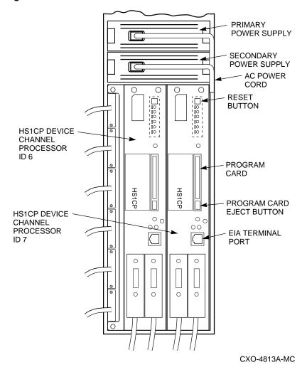
Figure 7–4 Device Channel Processor Installation
