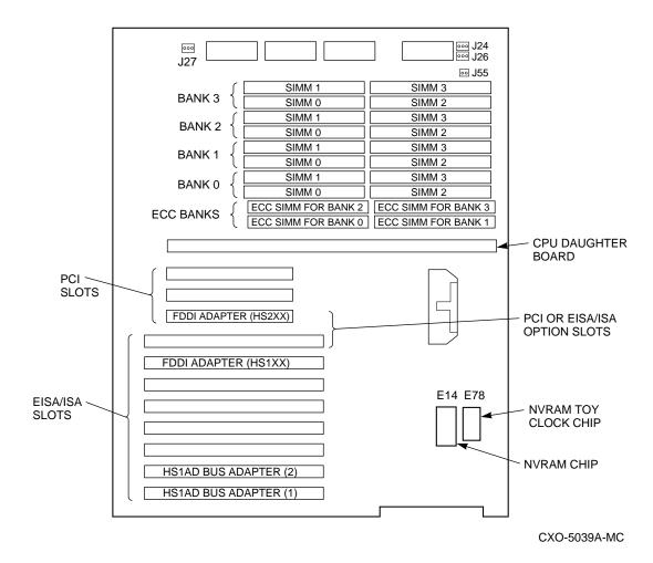
Figure 4–2 Server Processor Motherboard Configuration
