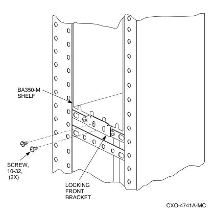
9. Once the shelf is positioned within the shelf mounting brackets, install the *locking front bracket* with 10–32 SEMS screws in the two middle holes as shown in Figure 3–13.
