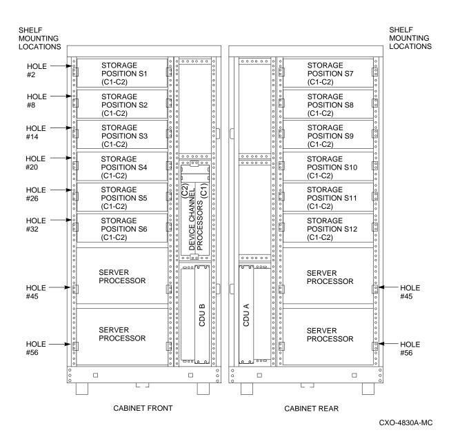
Figure 3–8 shows the location of storage shelves when disks but no TZ8*xx*–series tape drives are installed in a generalized FDDI Server.
