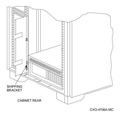
5. Install left and right shipping brackets at hole positions 53 and 54 on both *rear* vertical rails.
