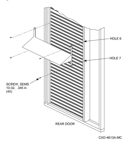
3. Install the horizontal air baffle to the rear door at hole positions 6 and 7 (from the top of the door) on both sides. Secure the baffle with  $10-32 \times .343$  inch SEMS screws. When the rear door is closed, the horizontal baffle slides over the vertical air baffle (see Figure 3–7).
