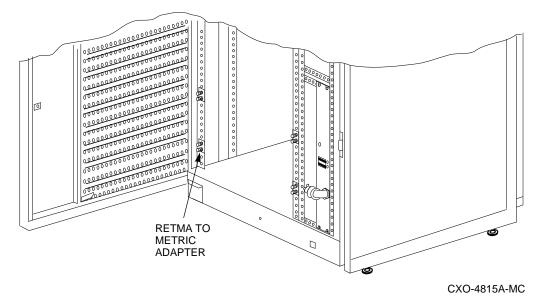
Figure 6–9 RETMA-to-Metric Slide Adapter Installation
