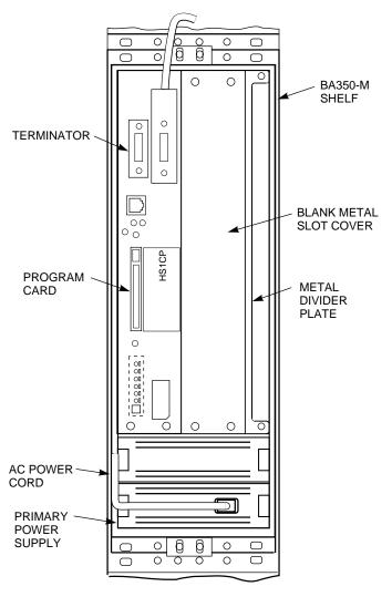
Figure 7–2 Single HS1CP Device Channel Processor in the Rear BA350–M Shelf
