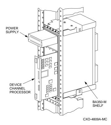
Figure 3–15 shows the installation positions of the power supply and device channel processor into the BA350–M shelf.
