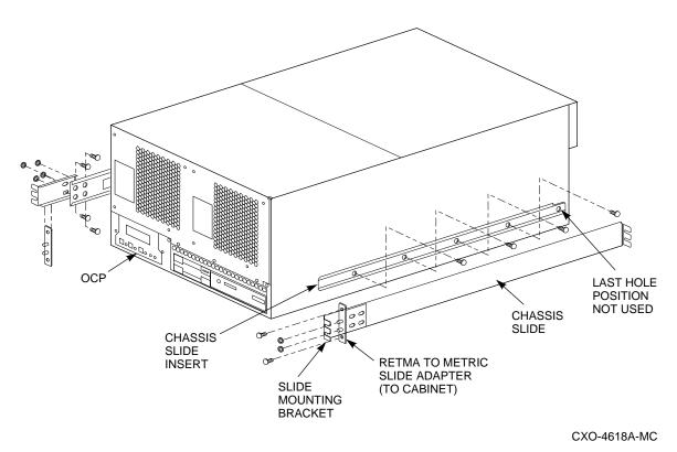
6. Remove the slide inserts from the chassis slide.
