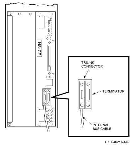
Figure 3–25 Trilink Connector with Cable and Terminator
