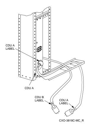
8. Use the hardware provided in the kit to mount CDU B to the cabinet chassis rails (see Figure 6–3).
