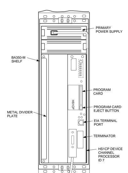
Figure 3–28 HS1CP Device Channel Processor
