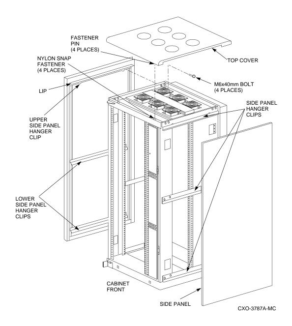
Figure 3–1 Exterior Cabinet Panel Removal (and Installation)
