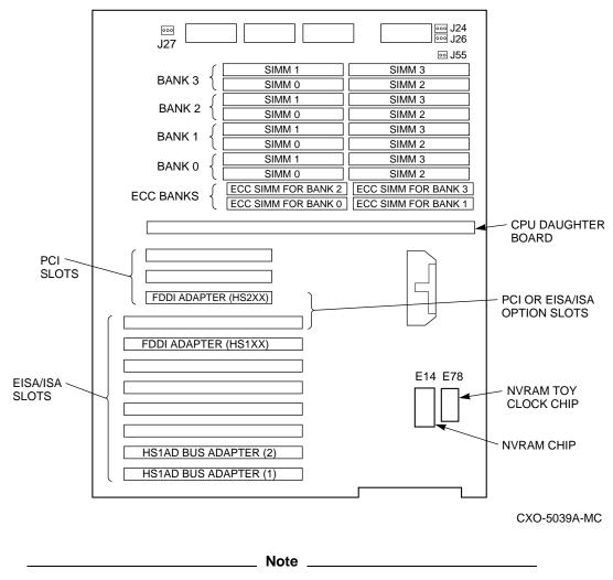
Figure 6–8 Slot Position for Device Bus Adapter
