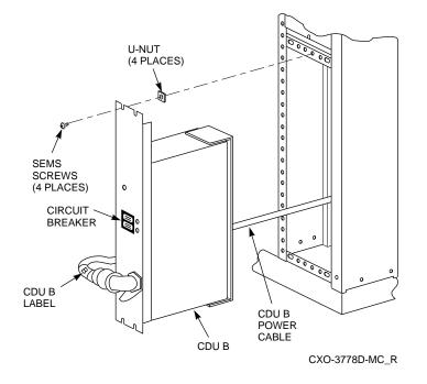
Figure 6–4 Rear Power Cord Installation
