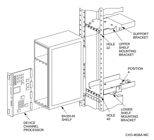
Figure 3–11 shows an exploded view of the components of the BA350–M shelf assembly:
