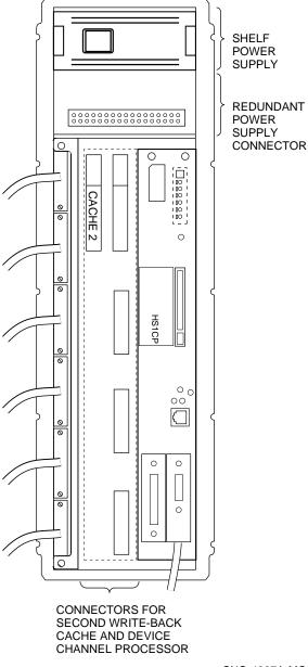
Figure 3–16 Slot 7 Device Channel Processor Installed
