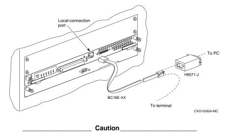
The local-connection port described in this book generates, uses, and can radiate radio-frequency energy through cables that are connected to it. This energy may interfere with radio and television reception. Don't leave any cables connected to it when you're not communicating with the controller.
