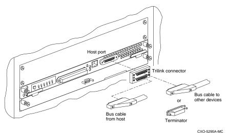
To connect a single, nonredundant controller to the host:
