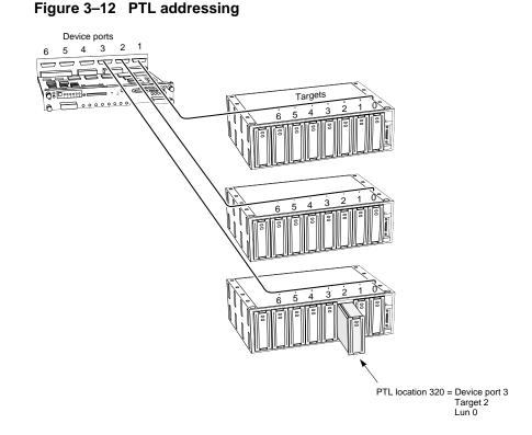
The controller uses the PTL location to name each device that you add to your subsystem with the CONFIG utility or CFMENU. (Factory-installed devices are added with the CONFIG utility. Thus, their names derive from their PTL locations.) For example, if the controller finds a disk in PTL 320, it names it DISK320; if it finds a tape drive at PTL 320, it names it TAPE320.
