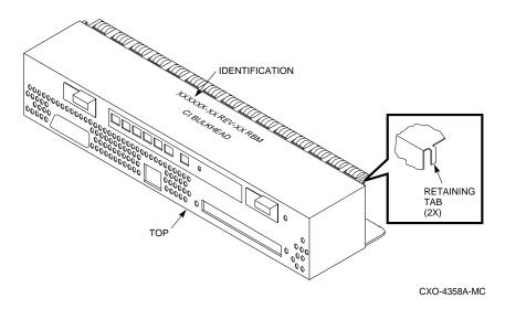
If you have an earlier controller (without identification or retaining tabs) you must snap the two retaining clips **9** to the outer corners of the cache module (on the edge furthest from the connector edge). The clips hold the module tightly in its slot and keep the weight of the batteries from dislodging the module.
