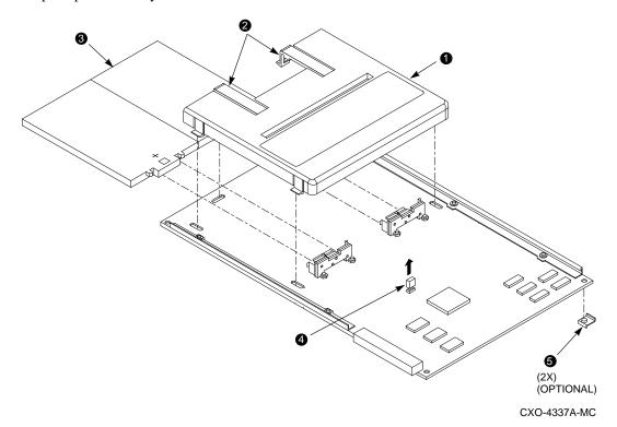
2. Disengage and gently lift the extended snaps ② on the plastic battery bracket and slide the batteries ③, positive (+) side up, straight into the module.
