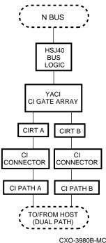
The CI interface for the HSJ-series controllers consists of a YACI CI gate array, and CI receiver/transmitter (CIRT) chips for the individual CI ports. The YACI gate array allows direct memory access of data between the host CI port and controller shared memory. Specialized host port firmware running on the policy processor sets up and maintains the CI port.
