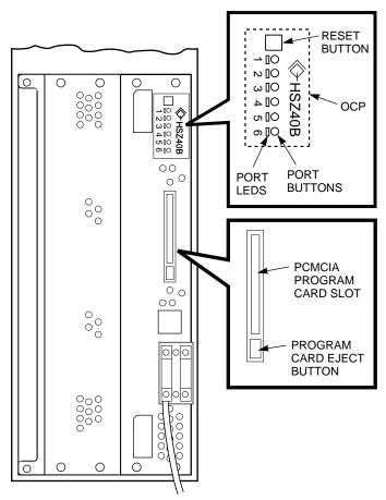
Figure 2–2 Operator Control Panel (HSZ-Series)
