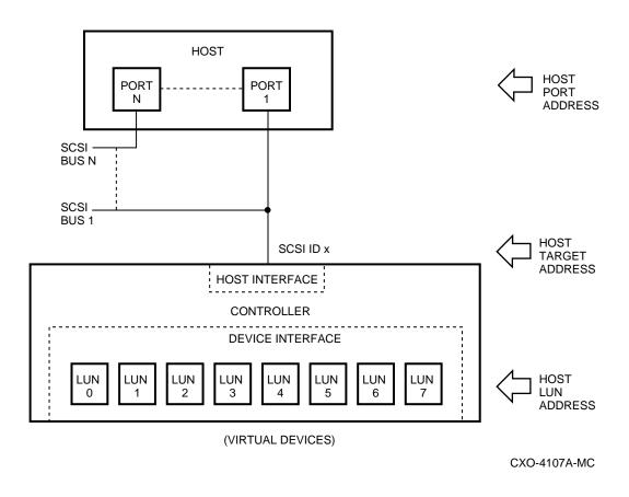
Although they share the same name, controller LUNs and SCSI host LUNs are names for two different storage structures. Controller LUNs exist on the *controller's* device interface, and SCSI host LUNs exist on a *host's* device interface.
