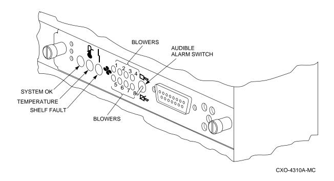
Table 5-4 EMU Control Panel LEDs/Switches and Error Descriptions
