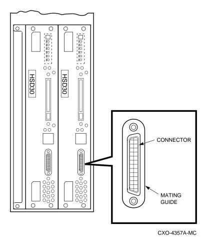
Figure 7-5 Trilink Connector (HSD- and HSZ-Series)
