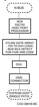
The DSSI interface consists of an NCR 53C720 chip plus specific DSSI logic and transceivers. The NCR 53C720 chip reads and runs scripts from controller shared memory to perform command and DMA operations on the DSSI interface. The policy processor sets up and maintains the operation of the NCR 53C720 chip.
