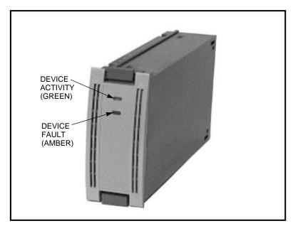
Figure 5-4 31/2-Inch Storage SBB LEDs
