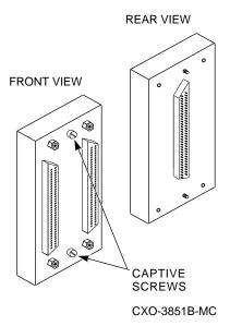
HSZ-Series: With a small flat-head screwdriver, loosen the captive screws on the trilink connector (see Figure 7-5) and remove the trilink from the front of the controller. Do *not* remove cables or terminators from the trilink, or you will interrupt the host SCSI bus. You will have to work around any SCSI cable or terminator connections when removing the trilink.
