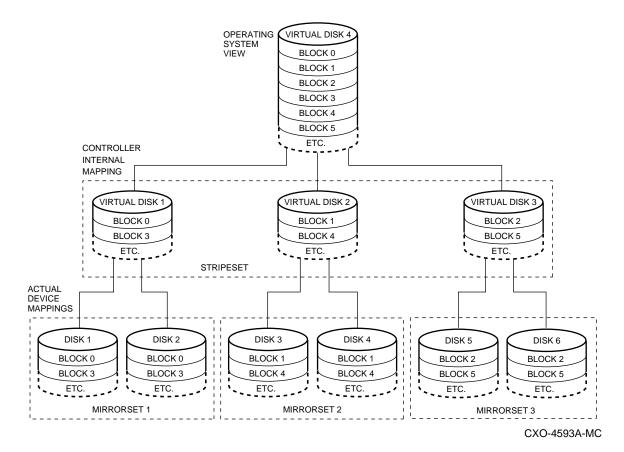
Mirroring is performed by the controller below the visibility of the host computer. Just as a host computer is not aware that a logical unit is actually a stripeset (as opposed to a single device), it also is not aware that a unit may be mirrored.
