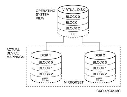
Mirroring requires the write-back cache module option to ensure data integrity. Both the write-back cache and mirroring are licensed firmware features.
