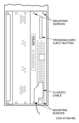
9. HSJ-Series: Loosen the captive screws on the CI cable connector, shown in Figure 7-3, with a flat-head screwdriver and remove the cable from the front of the controller module.
