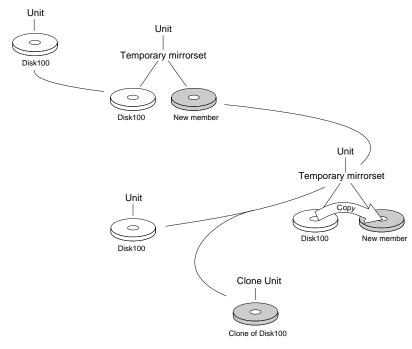
Figure 7–1 CLONE uses these key steps to duplicate each member of a unit.
