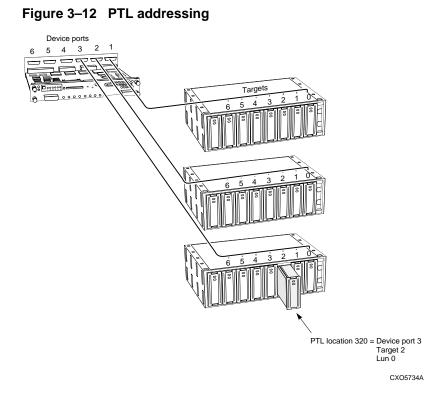
The controller uses the PTL location to name each device that you add to your subsystem with the CONFIG utility or CFMENU. (Factory-installed devices are added with the CONFIG utility. Thus, their names derive from their PTL locations.) For example, if the controller finds a disk in PTL 320, it names it DISK320; if it finds a tape drive at PTL 630, it names it TAPE630.
