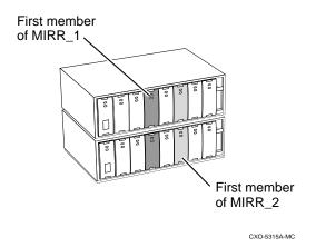
To avoid an I/O bottleneck on one bus, you can simply put the first members on different busses—in other words, put them in different shelves, as shown in Figure 3–5. Additionally, you can set the read-source switch to Round Robin. See *Read source* on page 3–19 for more information about this switch.
