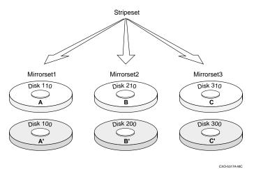
The failure of a single disk drive has no effect on this storageset's ability to deliver data to the host and, under normal circumstances, it has very little effect on performance. Because striped mirrorsets do not require any more disk drives than mirrorsets, this storageset is an excellent choice for data that warrants mirroring.
