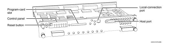
Under normal circumstances, you will not need to remove the controller from its cabinet. For this reason, the components that you will use most often are conveniently located on the front panel. For example, the localconnection port provides a convenient way to connect a terminal to your controller so that you can configure it for the first time.
