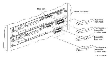
To connect a pair of multiple bus-failover dual-redundant controllers to the host:
