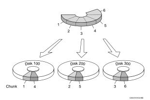
The relationship between the chunk size and the average request size determines if striping maximizes the request rate or the data-transfer rate. You can set the chunk size or let the controller set it automatically. See *Chunk size* on page 3–22 for information about setting the chunk size.
