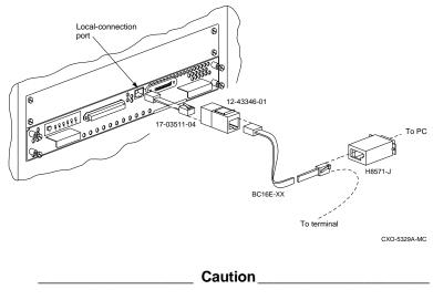
The local-connection port described in this book generates, uses, and can radiate radio-frequency energy through cables that are connected to it. This energy may interfere with radio and television reception. Don't leave any cables connected to it when you're not communicating with the controller.
