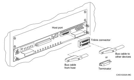
To connect a single, nonredundant controller to the host:
