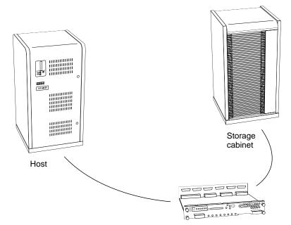
From the subsystem's perspective, the controller receives the I/O requests from the host and directs them to the devices in the subsystem. Since the controller processes all of the I/O requests, it eliminates the host-based processing that is typically associated with reading and writing data to multiple storage devices.
