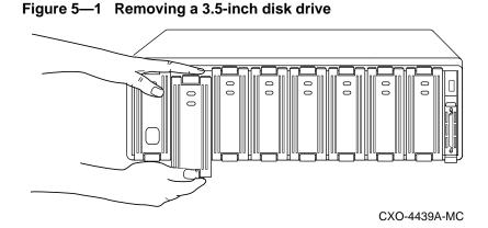
3. Using both hands, slide the disk drive out of the shelf and place it on flat surface (see Figure 5—1).
