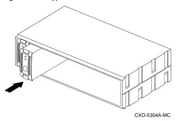
Figure 3—13 Typical 3.5-inch and 5.25-inch disk drive SBBs
