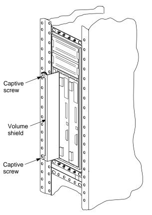
Figure 2–16 Removing the volume shield
