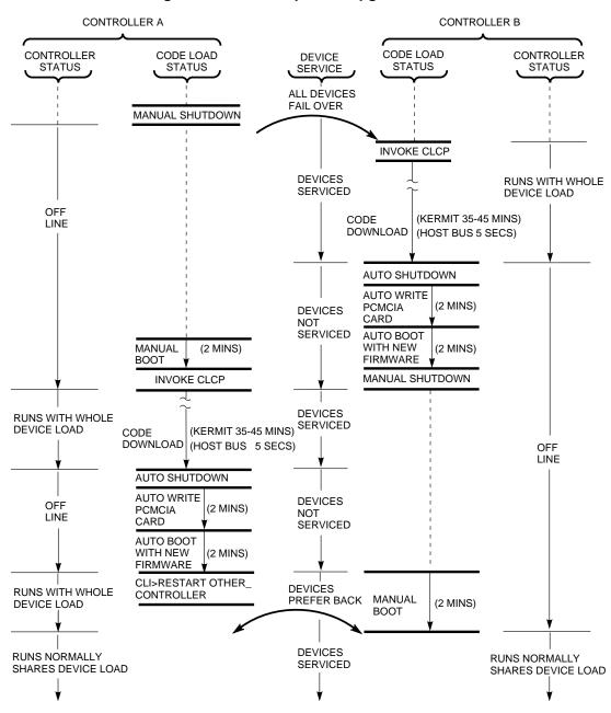
Figure 3—6 The sequential upgrade method
