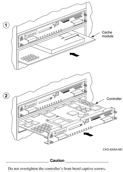
Figure 2–6 Installing the controller and cache modules
