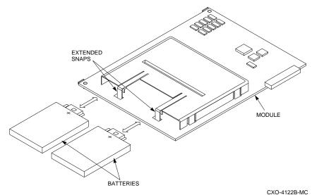
Figure 3—11 Installing write back cache batteries
