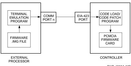
Figure 3—4 Terminal port code load operation
