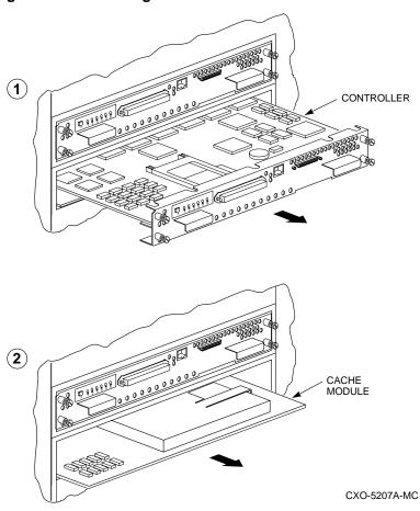
Figure 2–4 Removing the controller and cache modules
