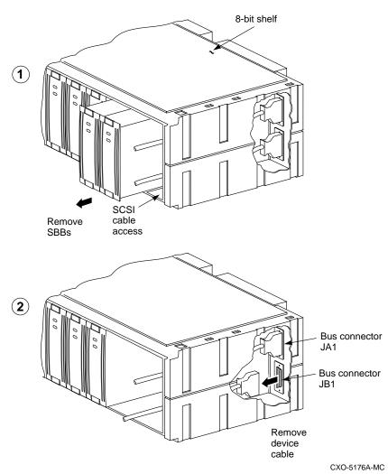
Figure 2–17 Access to the SCSI cables
