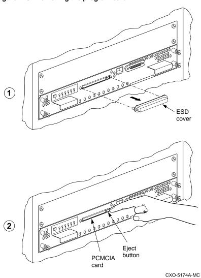
Figure 2–3 Removing the program card
