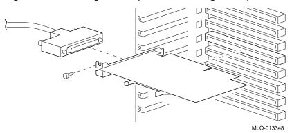
Figure 1–2 Installing KFPSA (End-Node Configuration)
