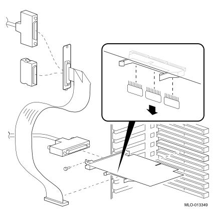
Figure 1–3 Installing KFPSA (Middle-Node Configuration)
