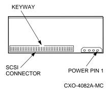
3. When the device connector is positioned with the keyway at the *bottom* as shown in Figure 3–7, fold the cable as shown in the callouts in Figure 3–9.
