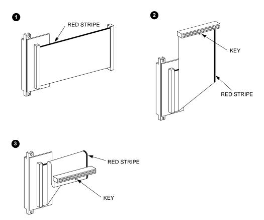
Figure 2–5 Cable Folding–Key at the Bottom
