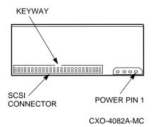
3. When the device connector is positioned with the keyway at the bottom as shown in Figure 2–3, fold the cable as shown in the callouts in Figure 2–5.
