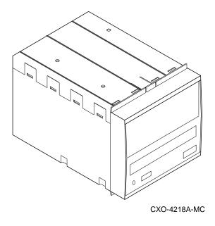
Figure 1–2 Maximum Full–Height Device Measurements
