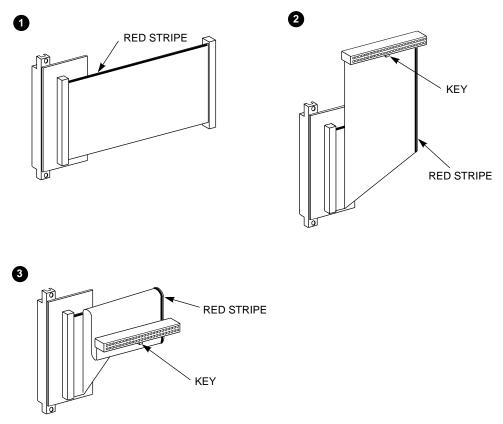
Figure 3–9 Inverted Device Connector Orientation
