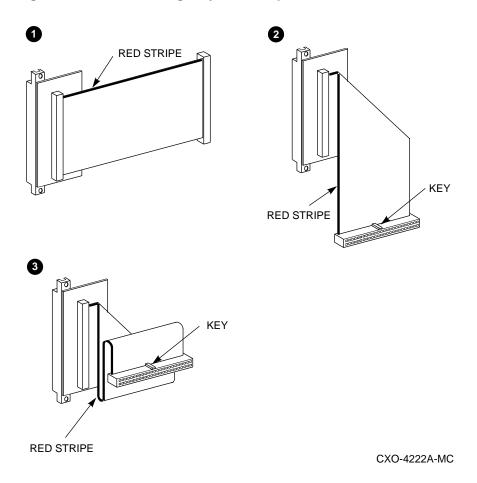
Figure 2–4 Cable Folding–Key at the Top
