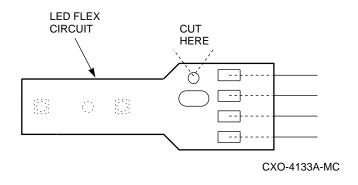
3. As shown in Figure 2–13, insert the upper right edge of the LED flex circuit under the upper right retaining tab on the back side of the fixed media device bezel.
