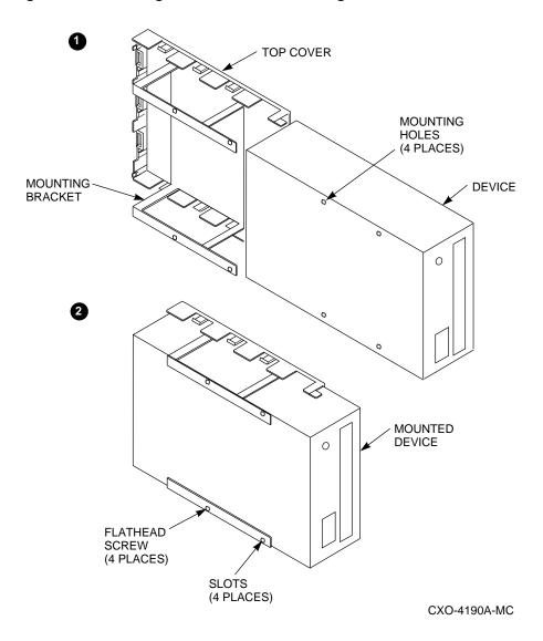
Figure 3–3 Installing a Device in the Mounting Bracket
