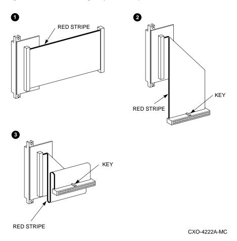
Figure 3–8 Cable Folding–Key at the Top
