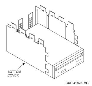
2. Place the bottom SBB cover on its side as shown in Figure 2–8.
