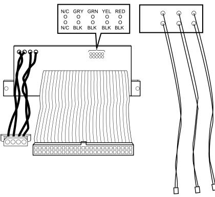
Figure 2–1 Connecting the ID Cable Harness
