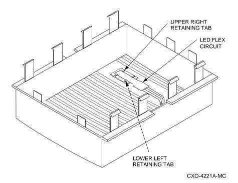
Figure 2–13 Fixed Media Device Bezel—Rear View
