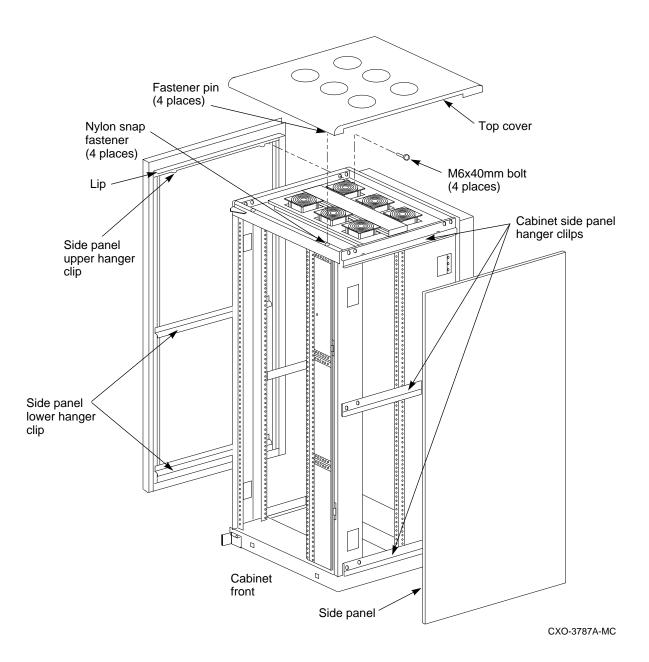
3. Using Figure 2–1 for reference, remove the side panels as follows:
