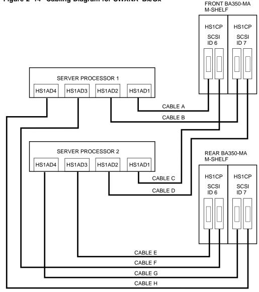
Figure 2–14 Cabling Diagram for SWXNA–Bx/Gx
