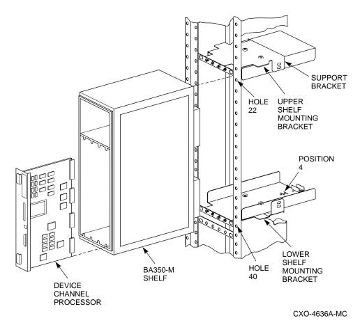
Figure 2–6 shows an exploded view of the components of the BA350–M shelf assembly:
