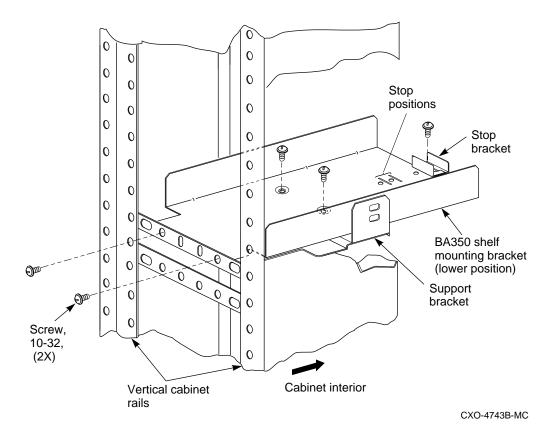
Figure 2–7 shows the proper horizontal cabinet bracket configuration for the *lower* BA350–M shelf mounting bracket.
