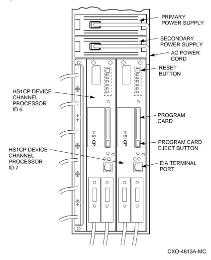
Figure 2–15 Device Channel Processor Installation
