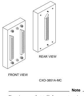
Exercise care that trilink connector pins are not bent or damaged when connecting an internal bus cable into a trilink connector.
