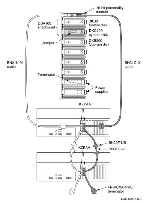
Figure 2–23 Shadowed System Disk Interconnection
