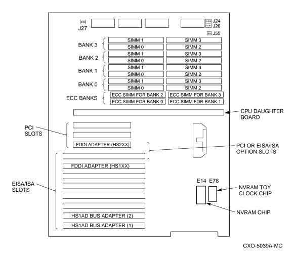
Figure 2–12 HS1XX Server Processor Motherboard Configuration
