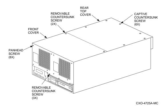
Figure 2–11 Removing the Rear Top Cover Panel
