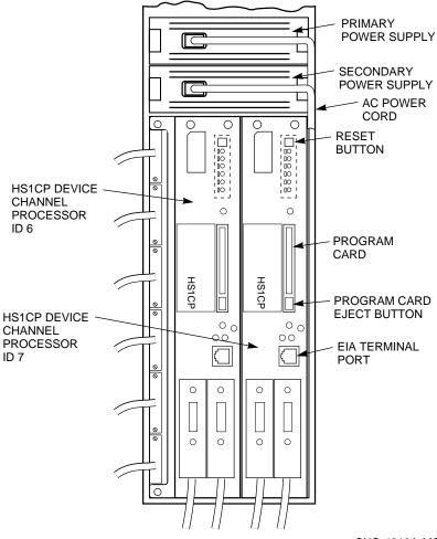
Figure 2–18 Device Channel Processor Installation
