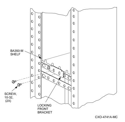
9. Once the shelf is positioned within the shelf mounting brackets, install the *locking front bracket* with 10–32 SEMS screws in the two middle holes as shown in Figure 2–8.
