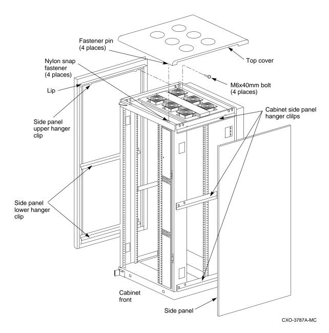
Figure 2–1 Exterior Cabinet Panel Removal (and Installation)
