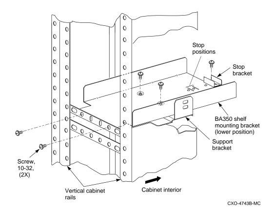
Figure 2–7 BA350–M Shelf Mounting Bracket Installation (Lower)
