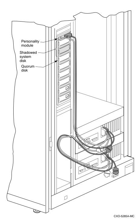
Figure 2–21 Shadowed System Disk
