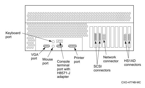
Figure 1–1 Connecting to the Terminal Port of the Network Array
