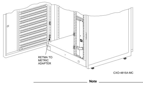
No adapter is needed on the *left rear* vertical rail of the cabinet, because the vertical air baffle has permanent mounting studs for the chassis slides.
