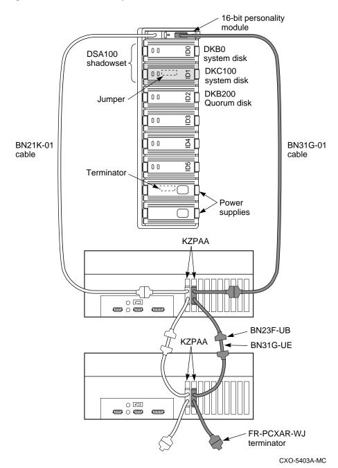
Figure 2–19 Shadowed System Disk Interconnection
