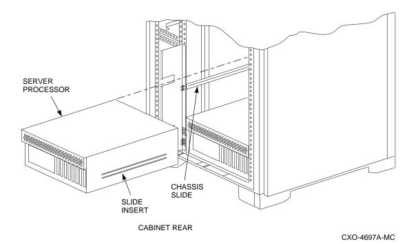
2. Slide the new server processor out of the front of the cabinet on its slides to easily access the rear top cover panel.
