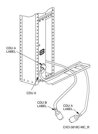
8. Use the hardware provided in the kit to mount CDU B to the cabinet chassis rails (see Figure 2–4).
