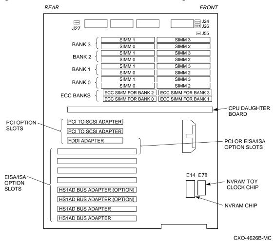
Figure 2–10 SWXNA Server Processor Motherboard Configuration
