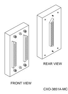
Some internal bus cable and terminator connectors do not provide enough access to the trilink screws for you to disconnect the trilink (without first disconnecting the cable and/or terminator). In these cases, you must disconnect power from all bus members and disconnect cables and terminators before disconnecting the trilink connector block.
