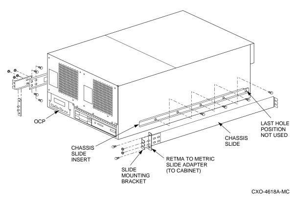
Position the slide insert so that the metal locking tab is outside and the <u>notch</u> on each slide insert is toward the rear of the server processor (see Figure 2–13). Align the screw holes on the server processor with the holes to the slide insert.
