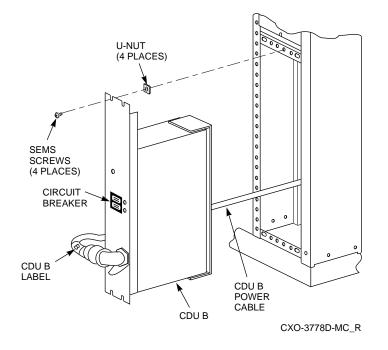
Figure 2–5 Rear Power Cord Installation
