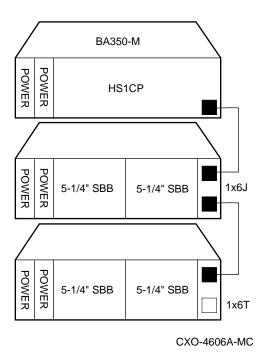
Figure B-2 is an example of two adjacent tape drives attached to a single port of the controller shelf.
