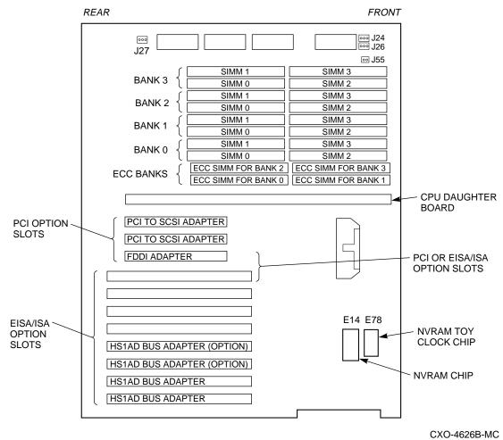
Figure 2-3 SWXNA Server Processor Motherboard Configuration
