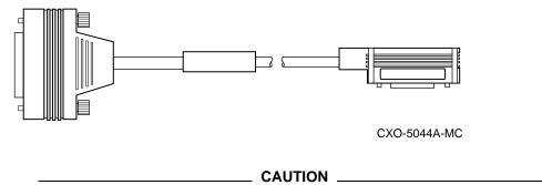
Currently, component damage can result if internal bus cables are connected or disconnected with power applied, unless the mating guide (Digital part number 74-49066-01) is installed around the outside edge of the HS1CP port connector. HS1CP modules are shipped from the factory with the mating guide and the trilink connector block premounted on the **HS1CP** port connector.
