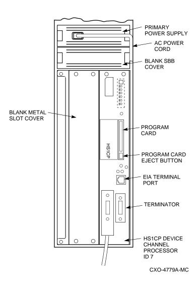
Figure 2–5 Blank SBB and Metal Slot Covers Installed
