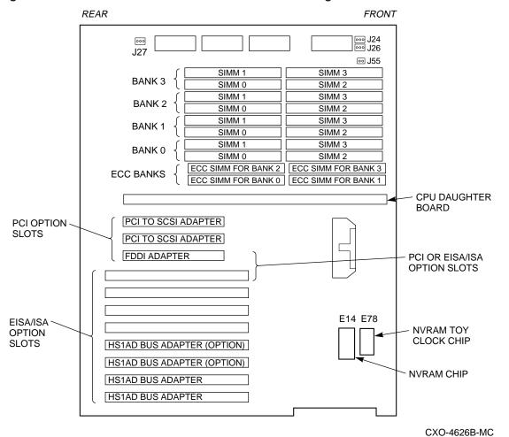
Figure 2–2 SWXNA Server Processor Motherboard Configuration
