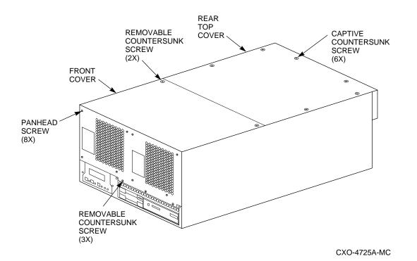
Figure 2–1 Removing the Rear Top Cover Panel
