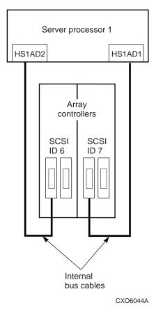
2. Plug a bus terminator into the other trilink connector on each HSD50 (see Figures 2–10 and 2–11). Figure 2–12 shows the BA350–M shelf with both HSD50 Array Controllers installed and cabled.
