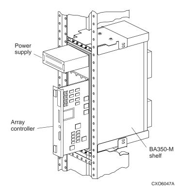
Figure 2–5 shows the installation positions of the power supply and array controller into the BA350–M shelf.
