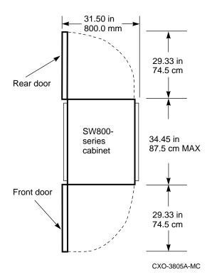
Figure 1-7 Minimum Installation Clearances
