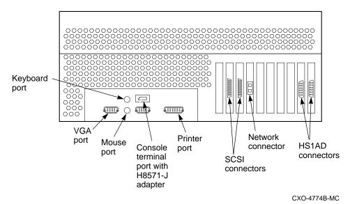
Figure 1–6 Connecting to the Terminal Port of the Network Array
