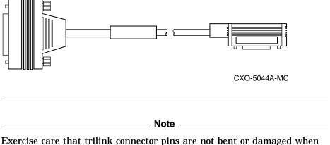
connecting an internal bus cable into a trilink connector.
