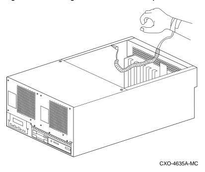
Do not disconnect the system unit power cord or unplug the power cord from the power supply socket. The power cord grounds the system, preventing damage to the internal components.
