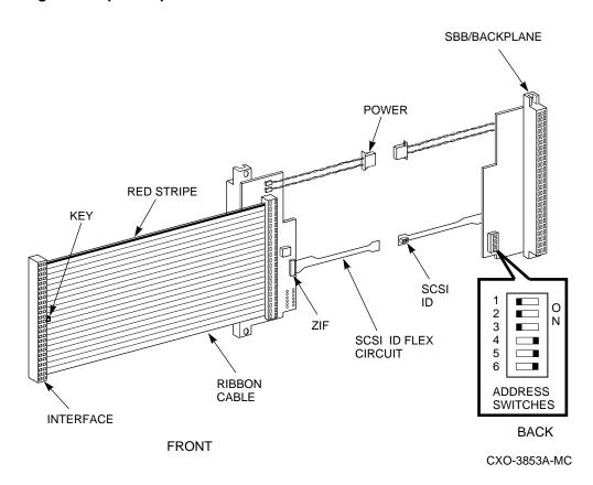
Figure 10 RRD42 Device Interface Connection
