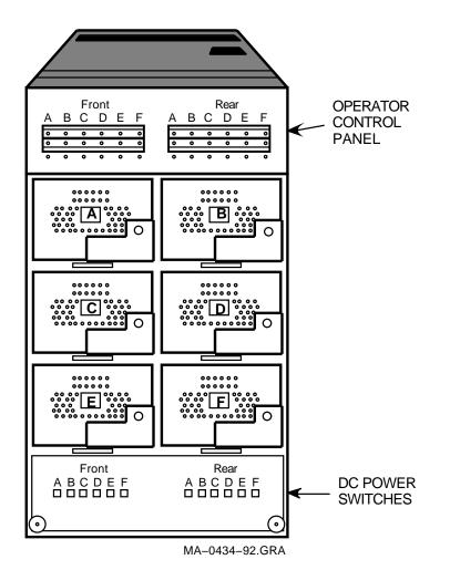
Figure 2–2 Front View of the SF3x Storage Enclosure (with cover removed)
