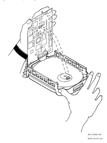
Figure 6–5 Separating the HDA from the Drive Module
