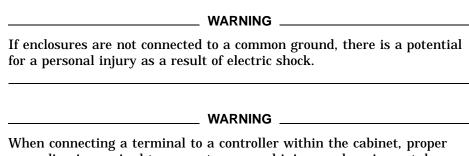
when connecting a terminal to a controller within the cabinet, proper grounding is required to prevent personnel injury and equipment damage. For optimum safety and performance, it is recommended that the terminal be powered by one of the two utility IEC outlets on the back of each cable distribution unit (CDU). A spare power cord is furnished with each cabinet for this purpose.
