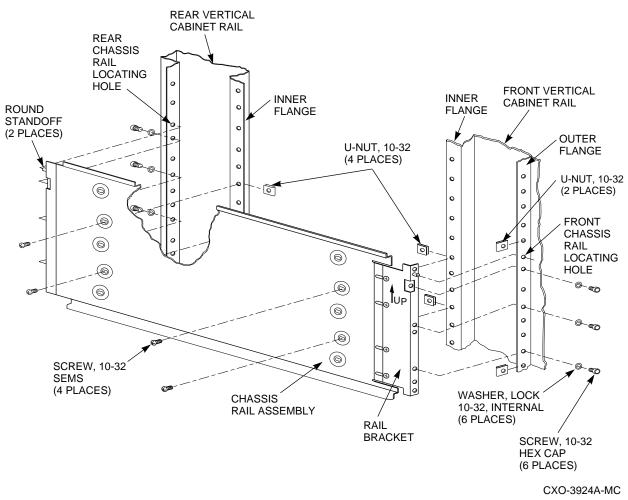
Use care in supporting the chassis rail assembly. It is heavy and awkward to position within the cabinet. If possible, use two persons to support and
