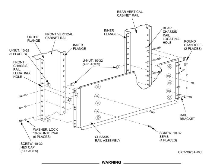
Use care in supporting the chassis rail assembly. It is heavy and awkward to position within the cabinet. If possible, use two persons to support and position the chassis rail assembly. The chassis rail assembly may cause personnel injury and equipment damage if dropped during installation.
