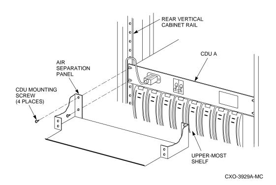
Figure 6-6 Rear Air Separation Panel Installation (Empty shelf position directly below CDU A)
