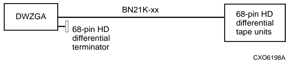
Figure 3-3 Remote DWZGA to 68-Pin HD Differential Tape Units
