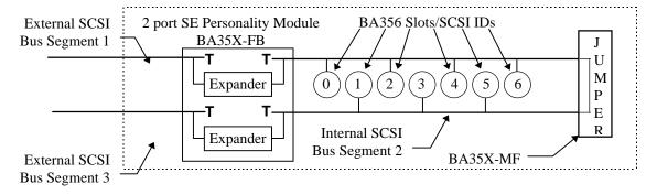
Figure 2 -- Personality Module Termination Scheme (Split bus)
