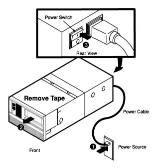
**NOTE:** If a tape had been left in the unit, it would be ejected on power-up, and should be carefully removed.
