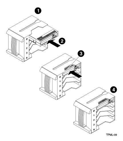
Figure 2–5 Inserting a Cartridge into the Magazine.
