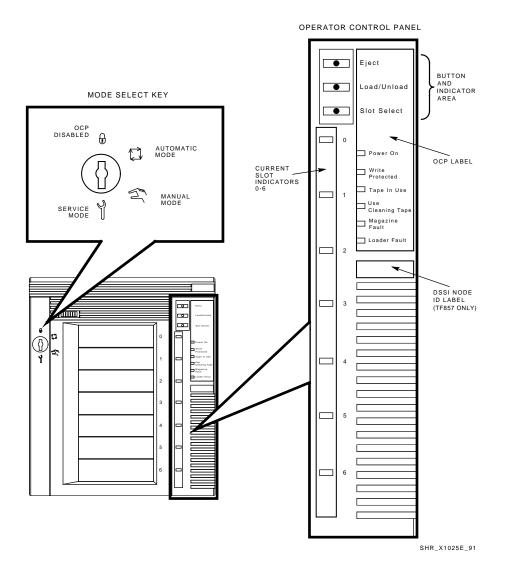
Operating Procedures 2–5 Using the Slot Select, Load/Unload, and Eject Buttons
