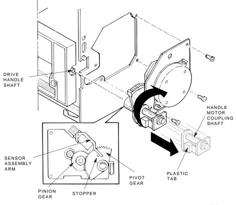
Figure 5–12 Handle Motor Assembly and Coupling Shaft
