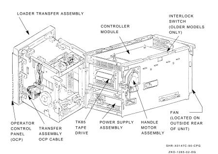
Figure 5–1 TF/TZ 800 Magazine Tape Subsystem FRUs
