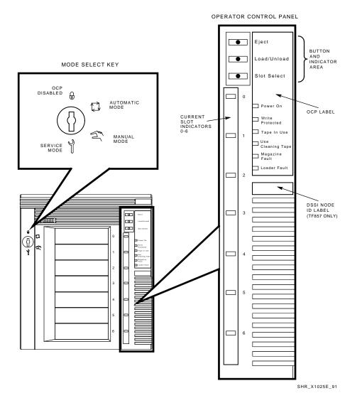
Firmware Update Procedures 8–5 TF85x Subsystem Firmware Update Procedure
