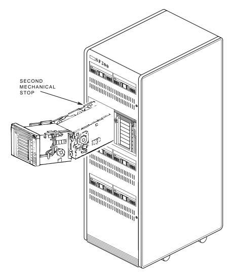
CXO-2461B SHR\_X1106C\_89 FRU Removal and Replacement Procedures 5–27 Removing and Replacing the TK85/TZ86 Tape Drive
