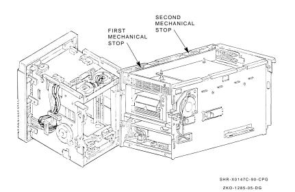
Figure 2–8 Mechanical Stops Associated with Service Mode (Older Modes)
