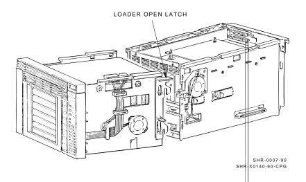
4. Open the receiver by squeezing the mechanical ejection lever (Figure 4–3) to remove the magazine.
