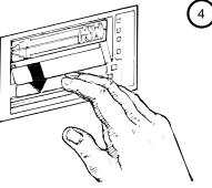
SHR-0256-87 SHR\_X1093\_89\_CPG Head Cleaning Procedure B–11 Inserting the CleaningTape III Cartridge into the Magazine
