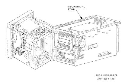
On models with two mechanical stops, the first stop lets you pull the front chassis forward from the enclosure to:
