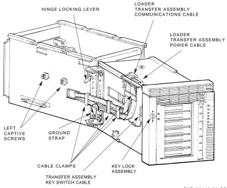
Figure 5–7 Left Side View of the TF/TZ 800 Subsystem
