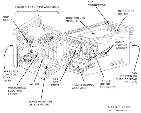
Figure 1–2 TF/TZ 800-Series Magazine Tape Subsystem Hardware Components
