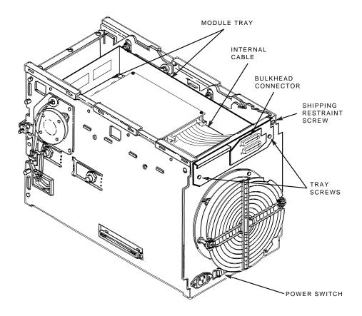
Figure 5–5 Rear Chassis with Components and Cables
