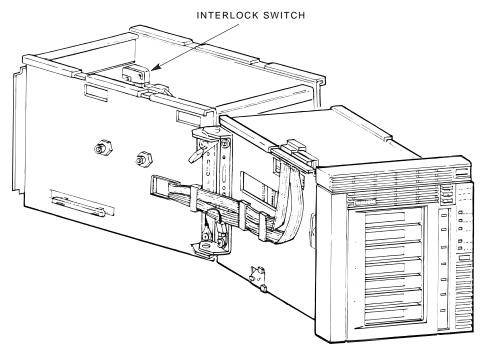
SHR-0009-90 SHR-X0143A-90-CPG 5–40 FRU Removal and Replacement Procedures Removing and Replacing the Power Supply Assembly
